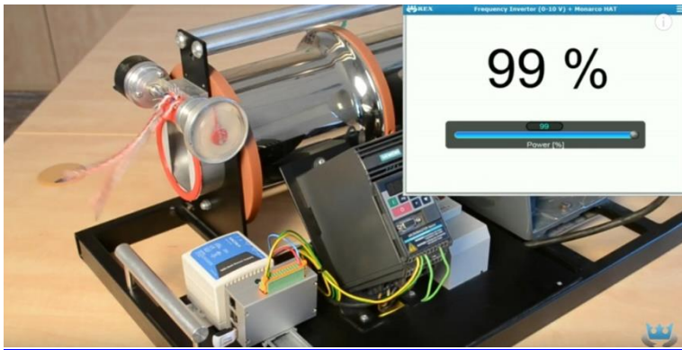
Attachment 3: Video demonstration: Raspberry Pi reading a 0-10 V ultrasonic sensor https://www.youtube.com/watch?time_continue=45&v=oXTaTk1jbEY
