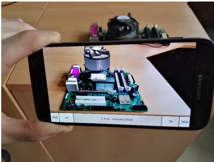
Fig. 8 Augmented reality work instruction
