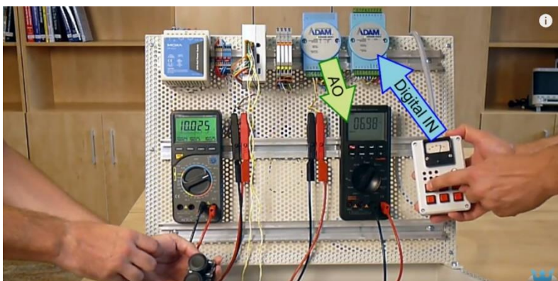
Attachment 4: Video demonstration: Extending I/O of the Monarco HAT via RS-485 https://www.youtube.com/watch?v=3G5M0xRgNss
