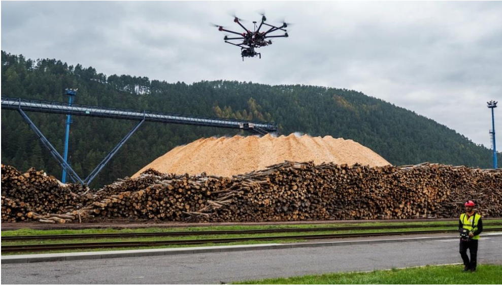
Fig. 6 – Volumetric Measurements by UAV
