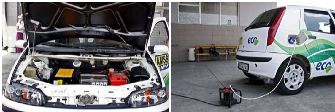
Figure 1-22 Converted FIAT Punto into e-car, “Zastava” company in Kragujevac
