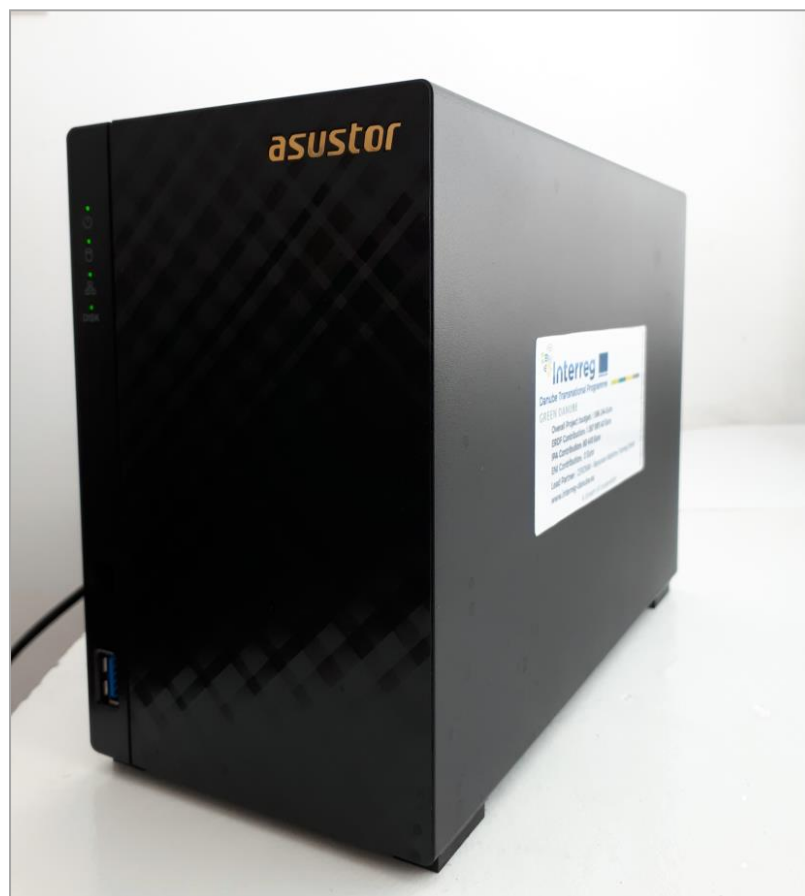
Figure 3.1: NAS Network Storage (2 x 2000 GB)
