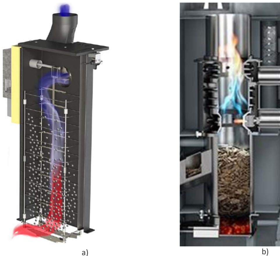
Figure 17: Example of developed solutions aimed to reduce pollutants emission, a) modular electric precipitator for flue gases b) solution of extreme staged combustion of wood pellets, with precise dosing of primary, secondary and tertiary air
