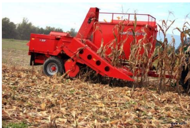
Figure 8: Corn ears picker-husker in operation
