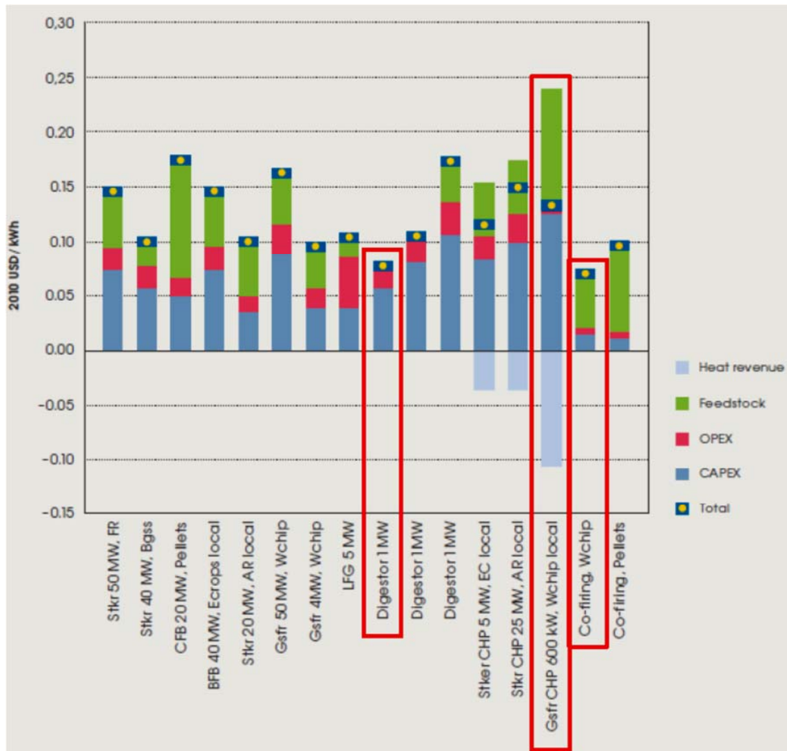
Figure 2: Levelized Cost of Energy for biomass technologies (Scarlat and Dallemand, 2017)
