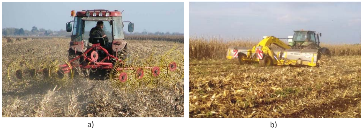
Figure: 9 Raking of shredded corn stover, a) finger-wheel rakes, b) wide pickup belt merger
