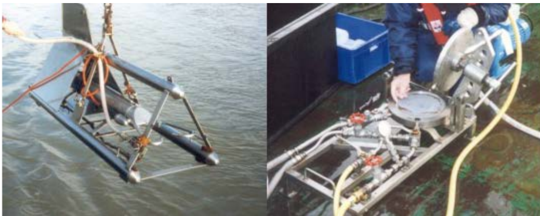
Figure 102 The Acoustic-Sand-Transport-Meter (ASTM) (left) and the filtering system that is used in The Netherlands to obtain fine-grained sediment samples (right) (BfG, 2008)
