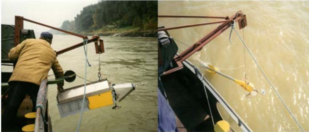
Figure 18 Measurements for the whole cross-section performed within the wider research programme on sediment transport using Ott-sampler and VUVH sampler (VUVH)
