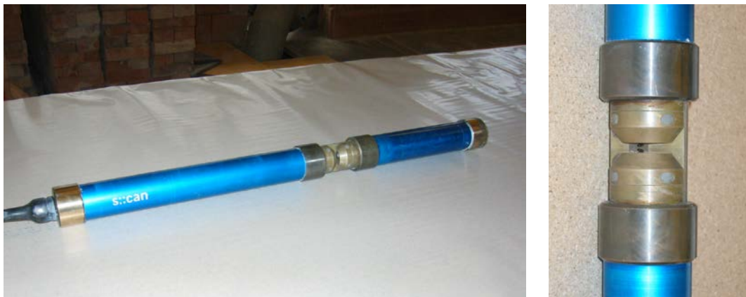
Figure 53 left: Spectro::lyser™ of s::can, right: optical path of Spectro::lysers (pictures: Bittner, 2008)
