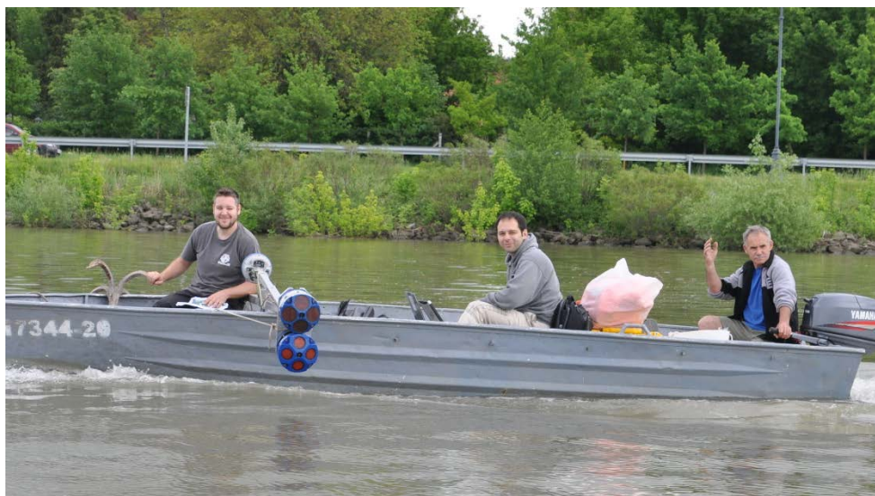
Figure 59 Parallel deployment of a 600 KHz and 1200 KHz ADCPs (photo: S. Baranya)
