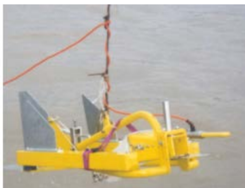
Figure 103 The Helley-Smith bedload sediment transport meter (BfG, 2008)
