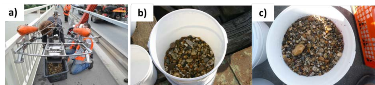
Figure 38 a: emptying the sampler after the measurement; b & c: bedload transport samples (IWHW/BOKU)
