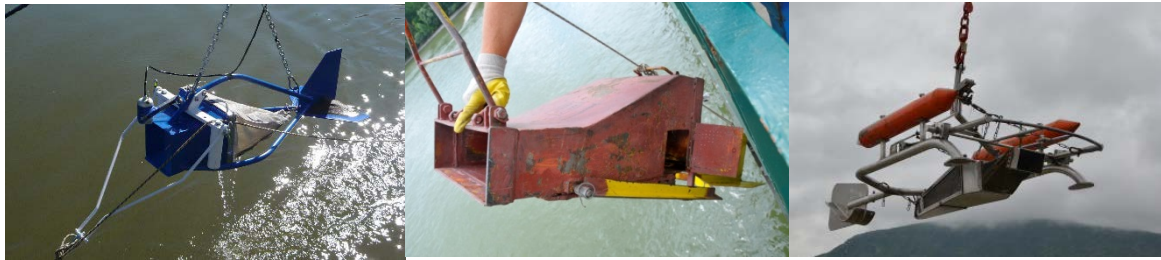
Figure 64 Pressure difference samplers – from left to right: Helley-Smith sampler, Karoly sampler and BfG-sampler (pictures by: Baranya/BME, Haimann IWHW/BOKU, Gmeiner IWHW/BOKU)
