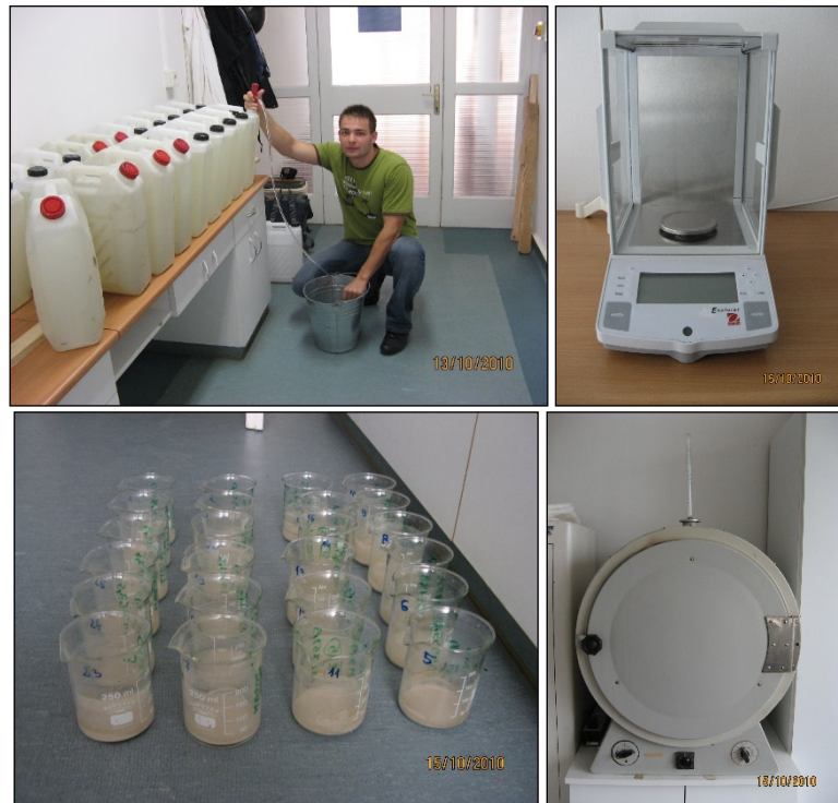
Figure 19 Laboratory analysis in Hungary. From left above: separation of clear water and settled suspended sediment; analytical balance; cups with dried material; oven
