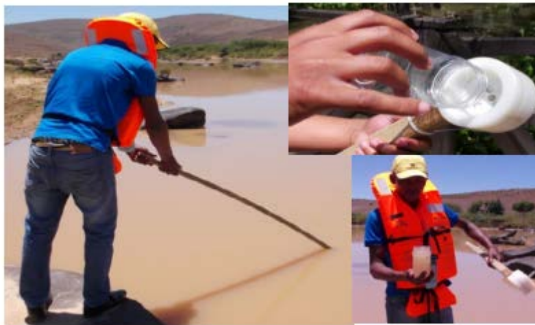
Figure 109 The wooden pole sampler in use showing the attachment of the sample jar into the head assembly
