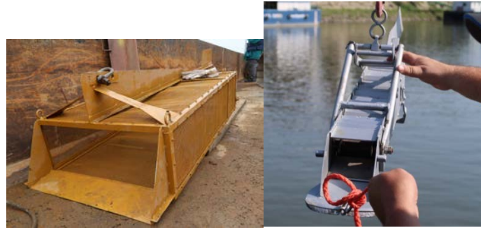
Figure 85 Basket samplers – from left to right: Sampler in use by the VUVH (SK) and sand bed sampler in use by NIHWMM (RO (pictures: Gmeiner / IWHW-BOKU)
