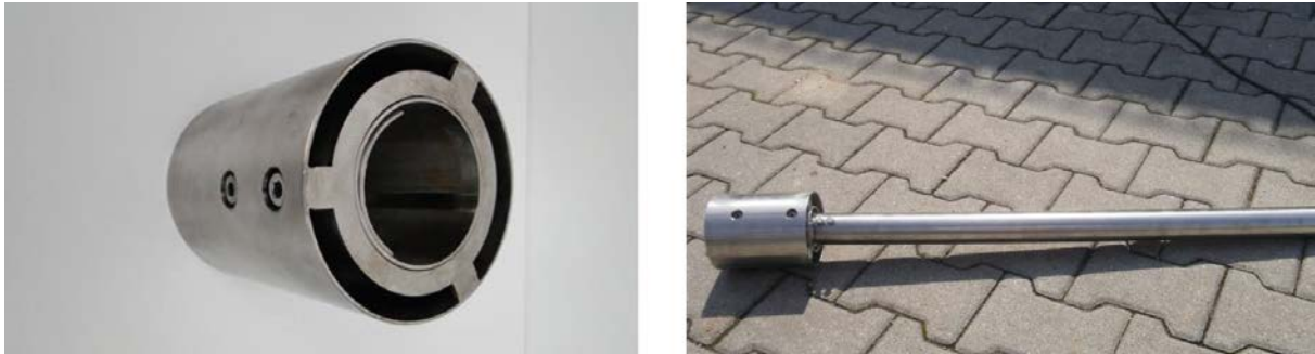
Figure 5 Protection case for Solitax ts-line optical backscatter (LfU, 2012)
