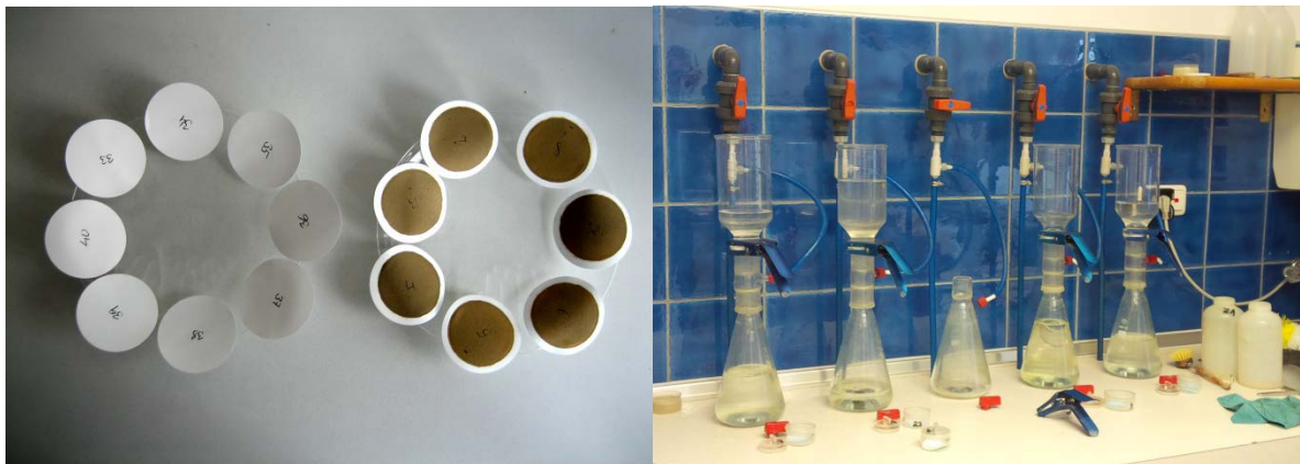
Figure 79 a) Membrane filter; b) Filtering of samples at the laboratory of viadonau in Aschach (pictures Haimann IWHW/BOKU).
