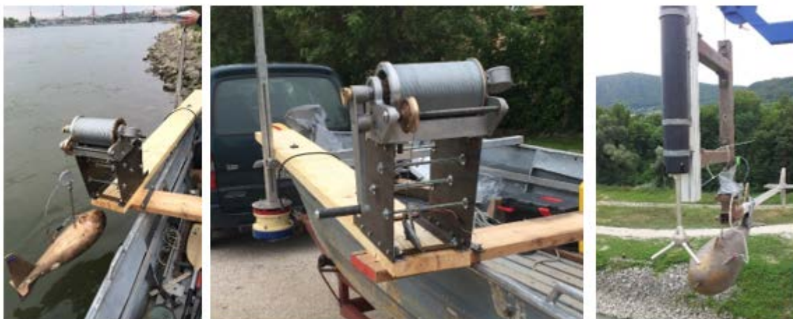
Figure 94 Measurement setup for suspended sediment sampling.
