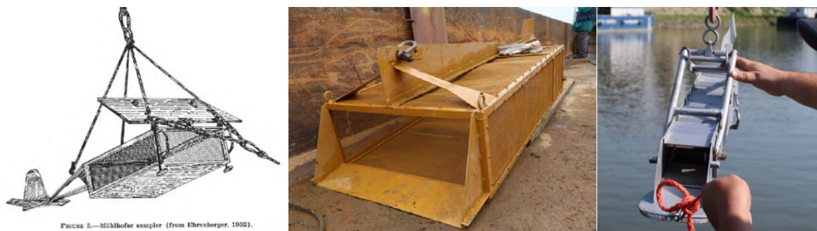
Figure 63 Basket samplers – from left to right: Mühlhofer sampler (Hubbell, 1964), sampler in use by the VUVH (SK) and sand bed sampler in use by NIHWM (RO).
