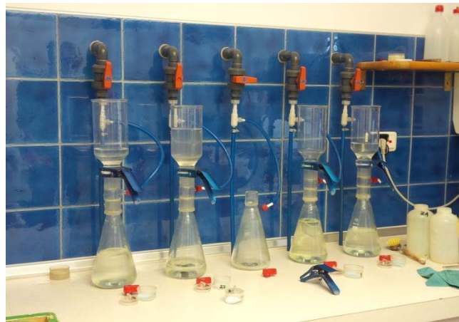
Figure 13 The vacuum filtration equipment in the laboratory (IWHW/BOKU)
