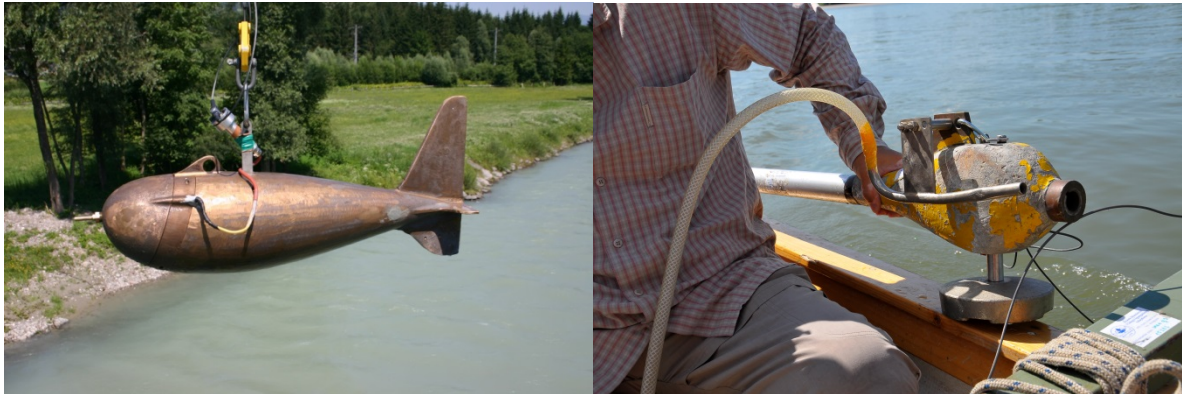
Figure 75 Suspended sediment samplers: a) US P61 A1 type sampler (BMLFUW, 2008; 2017); b) pump sampler (picture Haimann IWHW/BOKU).
