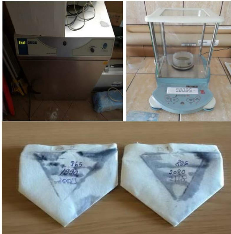
Figure 30 Oven; balance; dry and weighed filters
