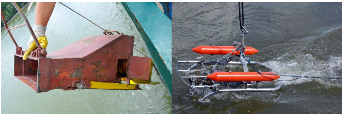
Figure 84 Cross-sectional Bedload samplers: Károlyi-type sampler (left (picture: Haimann / IWHW-BOKU); modified BfG sampler (right (picture: Liedermann / IWHW-BOKU))
