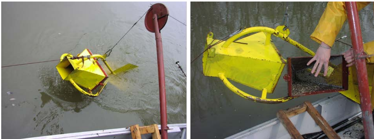
Figure 41 Helley-Smith sampler (modified by VUVH)
