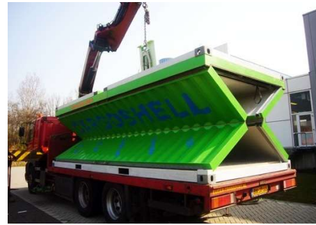
Figure 21 – Collapsible Shipping Container Source: TrendHunter 2018
