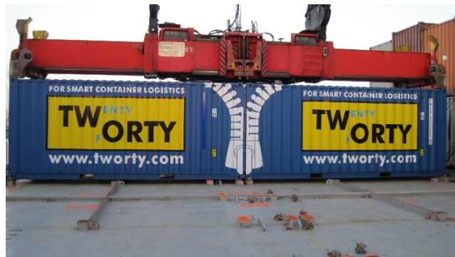
Figure 19 – Tworty Box in a 40-foot configuration Source: Container Technology Magazine 2017
