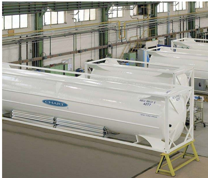
Figure 9 – LNG ISO container Source: Chart Industries
