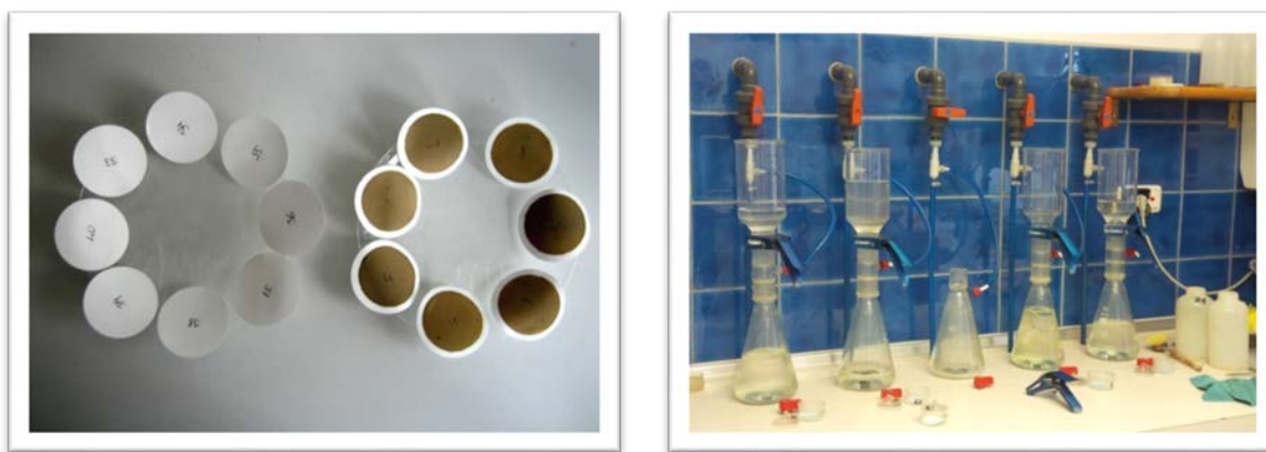
Figure 8 Membrane filter (left); filtering of samples at the laboratory of viadonau in Aschach (right) (pictures: IWHW/BOKU).
