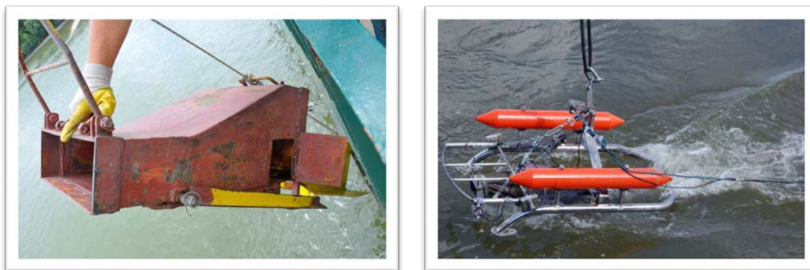
Figure 13 Bedload samplers: Károlyi-type (left); modified BfG sampler (right) (IWHW/BOKU).
