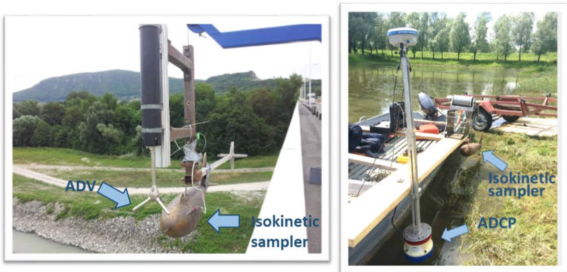
Figure 6 Setup of parallel sediment sampling and flow velocity measurement (left: IWHW/BOKU, right: BME)
