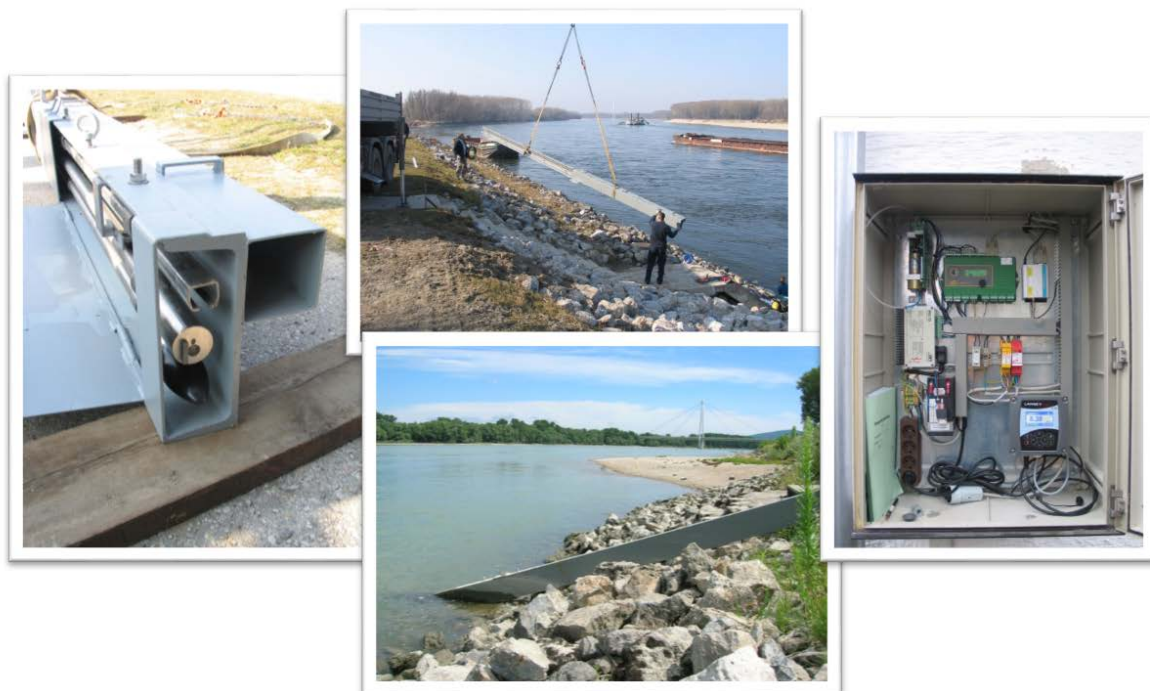
Figure 4 Turbidity sensor mounted on the river bank (source: viadonau)
