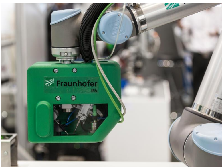
Figure: A safe soldering unit feasible for robot-human interactions
