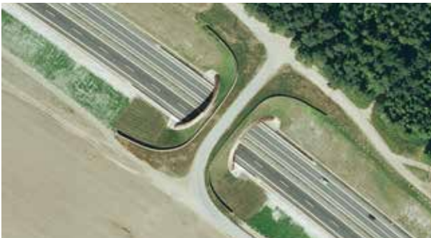
Fig. 6.34 Multipurpose use of bridges is usually the preferred solution in terms of costs. Also, linking functions of fauna passages with bridges over watercourses or with viaducts is suitable. On the contrary, a busy path on a green bridge can cause large mammals to avoid it, which then makes the entire measure non-functional. Poprad, Slovakia. © EUROSENSE s.r.o., 2010
