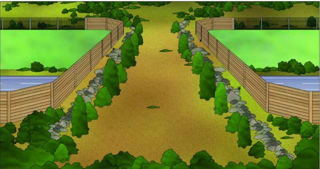
Fig. 10.22 General scheme of a green bridge. Such a fauna passage must always be equipped with barriers that eliminate noise, light and other disturbances, vegetation should be situated mostly along the sides, whereas the middle of the structure should stay open. © Spain, Ministry for Ecological Transition, 2016. Technical prescriptions for wildlife crossing and fence design (second edition, revised and expanded) (on line). Madrid: MAPAMA. Illustrations made by Pep Gaspar, ARTENTRAÇ
