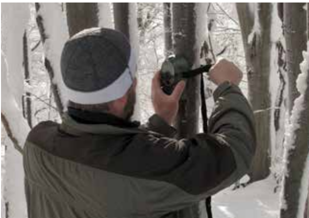
Fig. 12.12 The most common method in assessing the efficiency of fauna passages is the use of phototraps. They must be installed not only in the passage itself, but also in its surroundings. This enables to verify which animals have not used the passage. © Michal Kalaš
