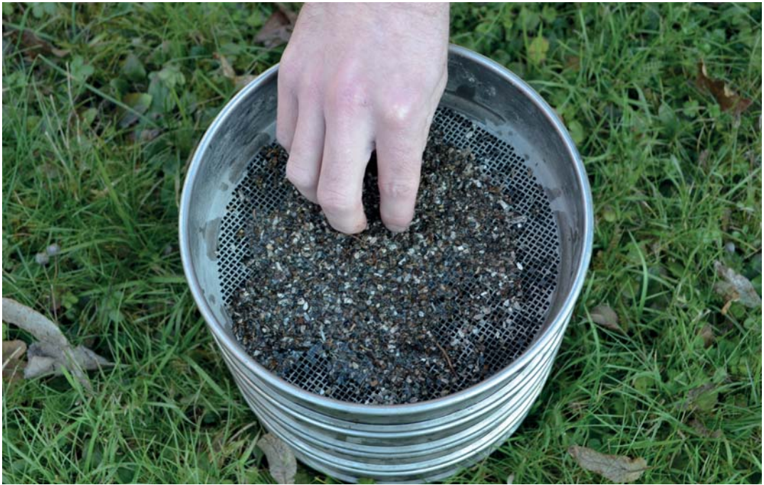
11.4.7 Figure 1: Wet sowing. The sediment is rinsed through the sieve(s) with a gentle spray of tap water delivered through a shower head. The spray must be strong enough to wash the finest material through the sieve, but not so strong as to damage delicate fossils (photo: University of Ljubljana, archive).
