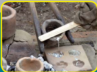
Casting a tin-alloy object with an Iron Age motif from Kleinklein (Styria, Austria)
