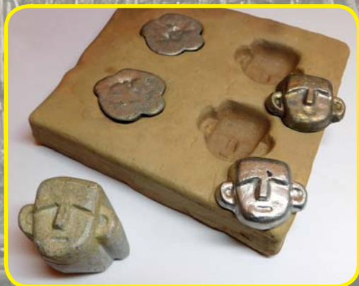
The ceramic mould and the form stamp, and the cast objects with an Iron Age motif from Kleinklein (Styria, Austria)
