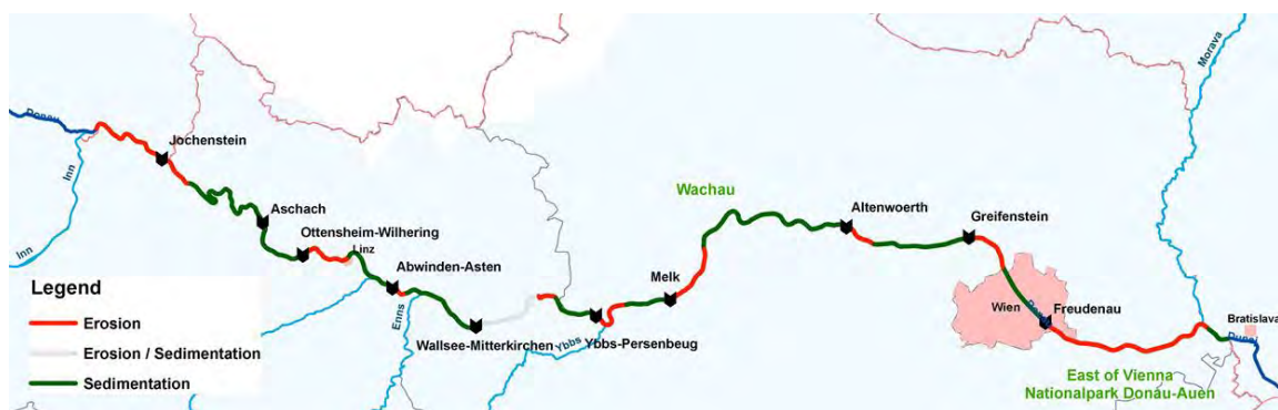
Figure 5.1.35 Classification of erosion and sedimentation in different parts of the Danube in Austria. Bathymetry, including dredging and feeding. Segments from the first measurement to 2001 for the Freudenau HPP since 1998.
