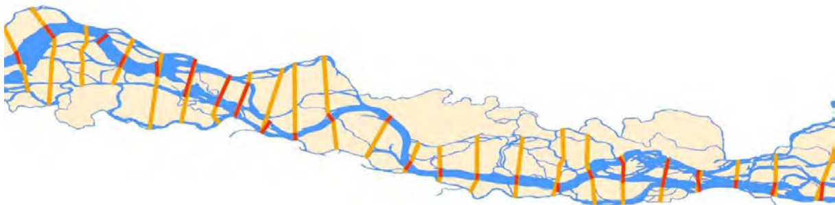
Figure 4.2.3 Estimation of the Danube river widths of the active channel (red colour) and of the river system (orange colour) for reference state
