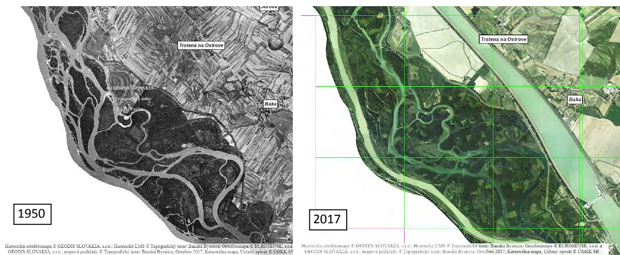
Figure 5.1.85 Satellite images of anabranching section of the Danube between Bodíky -Baka from 1950 and 2017 illustrate a successive degradation of the anabranch system (SK-HU area) (Source: GEODIS SLOVAKIA, s.r.o., © Topografický ústav Banská Bystrica, © EUROSENSE, s.r.o., © TU Zvolen)
