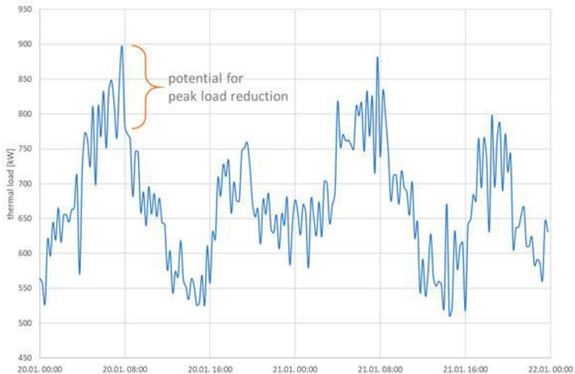
Figure 4.4.11: Thermal load course of the district heating grid in Strem from 20.01.17 to 22.01.17 including the potential for peak load reduction following DSM-measures
