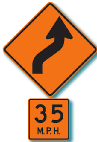
Figure 5. Horizontal curve warning sign with speed advisory plaque.
