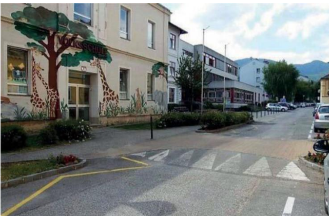
Yellow-paved elevation of road surface
