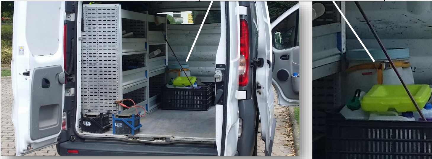
1. 30L PLASTIC TANK FIXED IN VEHICLE FOR TRANSPORT
