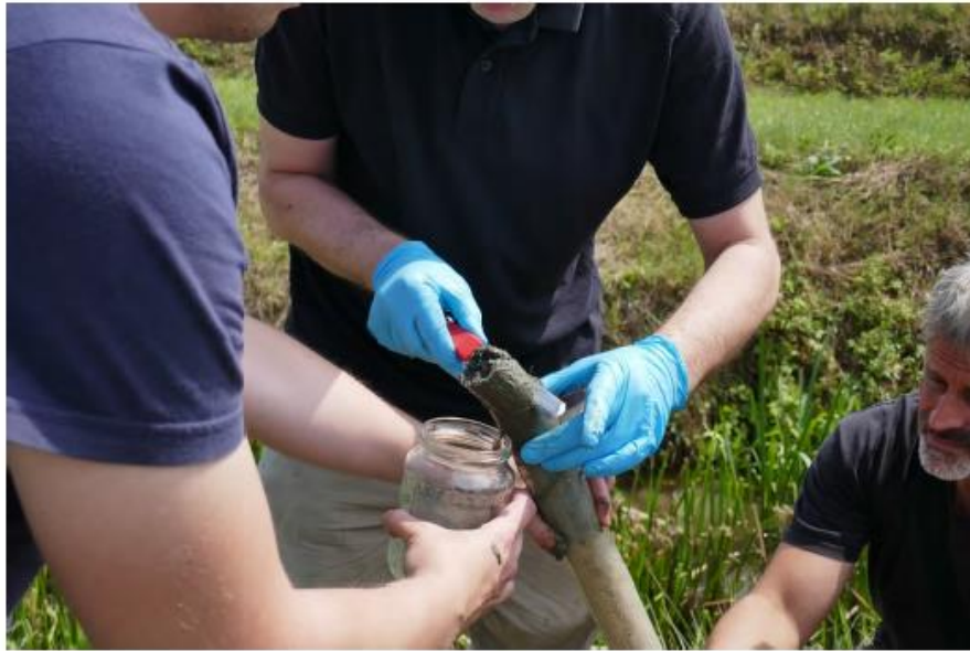
Figure 36. Pushing out the top 5 cm of bottom sediment with vacuum core system
