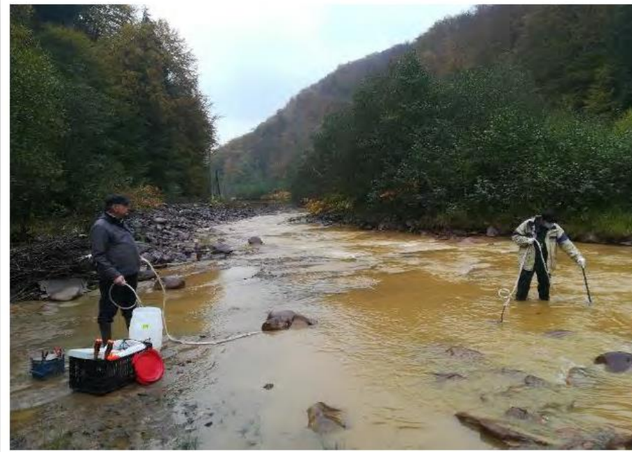
Figure 18: Suspended sediment collected into a 30 L barrel with underwater pump
