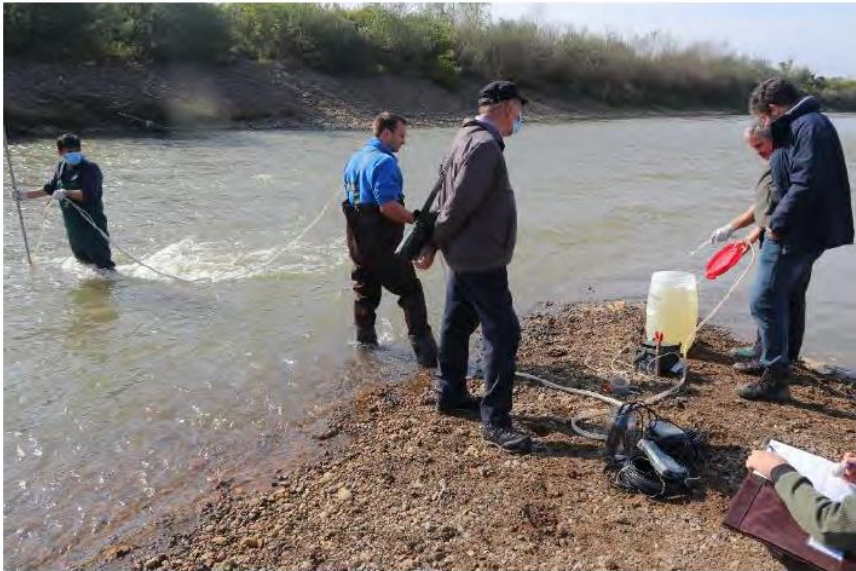
Figure 1.3. Suspended sediment collected into a 30 L barrel with underwater pump
