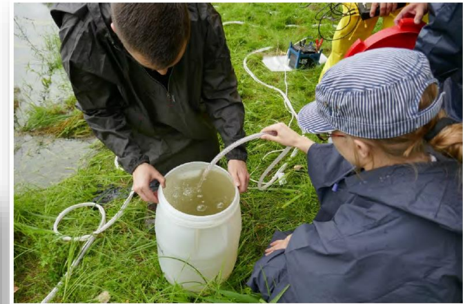
Figure 18: Suspended sediment collected into a 30 L barrel with underwater pump
