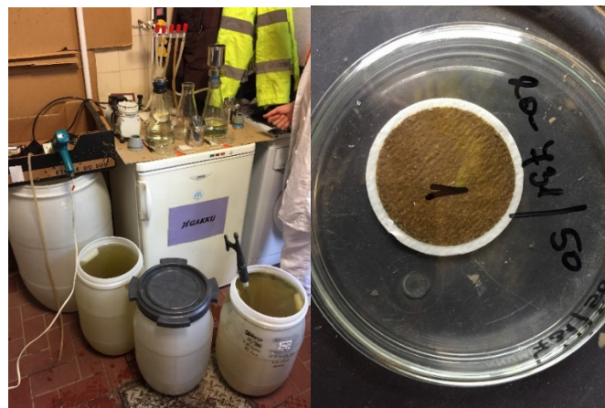
Figure 5. Suspended sediment samples pumped and filtered through a 0.45 \mu\text{m} filter (left) in the laboratory. Suspended sediment collected on the filter, ready for chemical analysis (right).
