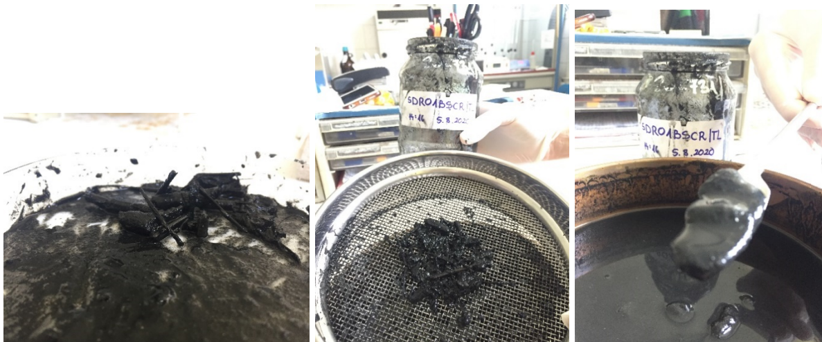
Figure 7. Stream bottom sediment samples contained plant fragments (left) that are removed by sieving to <2mm sieving (middle). The <63µm fraction fine mud (right).
