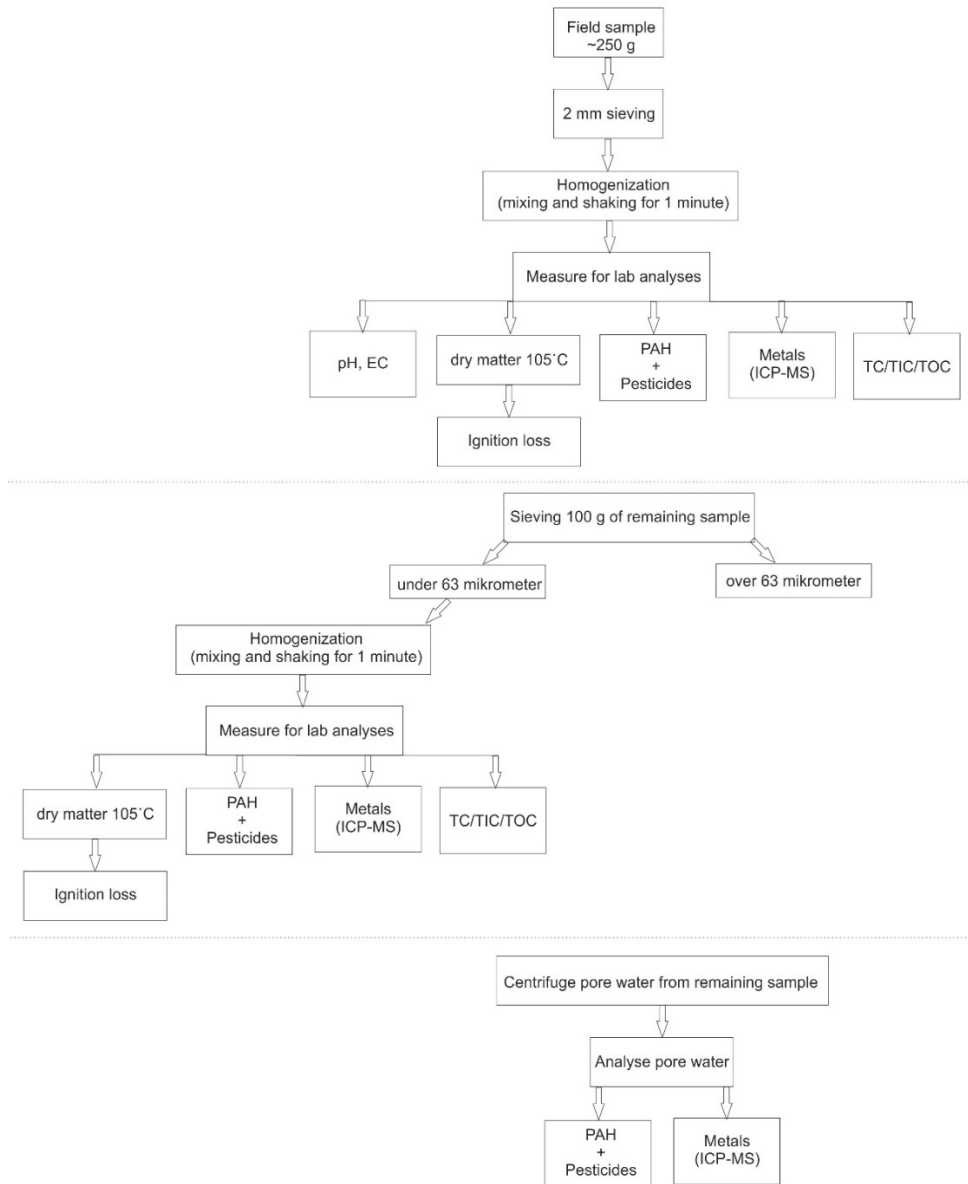
Figure 3. The scheme for sample preparation and analysis of stream bottom sediment samples.
