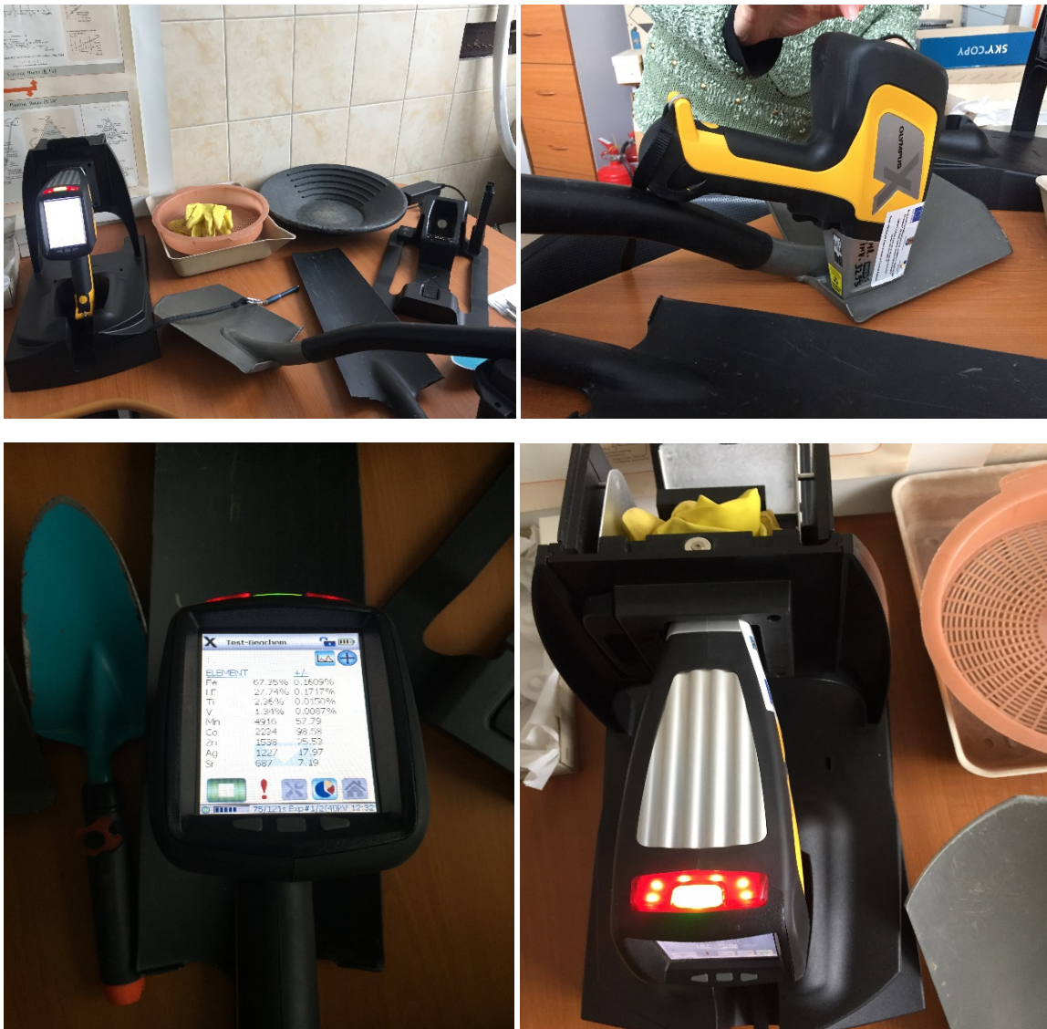
Figure 6. Testing the chemical composition of sampling tools using a portable XRF device in IGR-RO (the six photos above)
