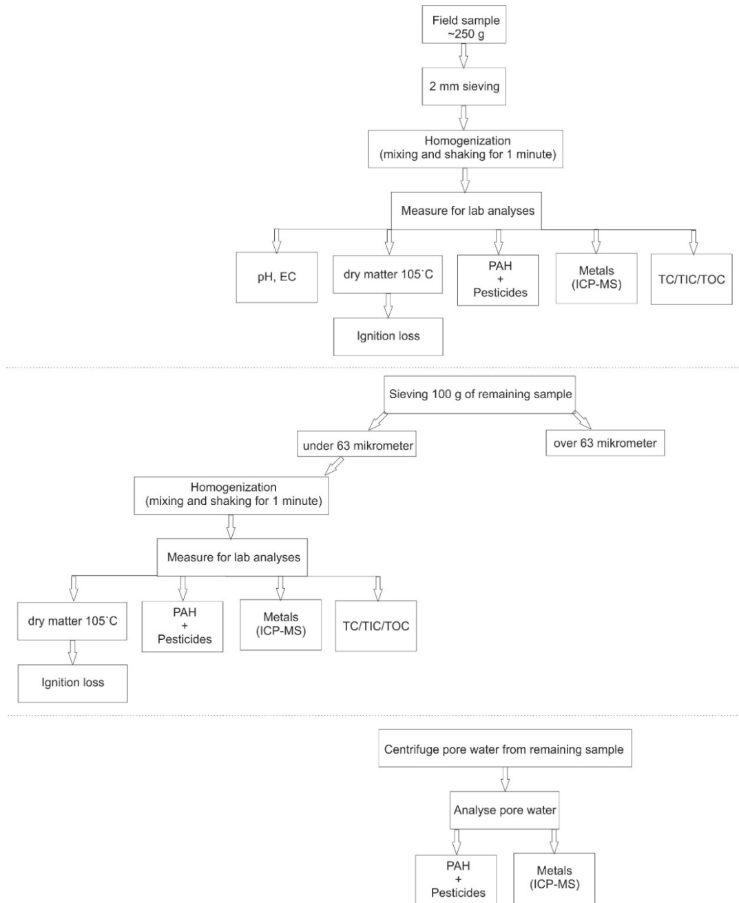
Figure 9. Final scheme for sample preparation and analysis of stream bottom sediment samples.
