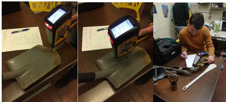
Figure 5. Testing the chemical composition of sampling tools using a portable XRF device.
