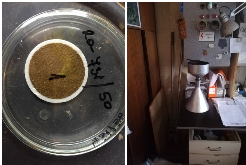
Figure 6. Suspended sediment samples pumped and filtered through a 0.45 \mu\text{m} filter (top pictures) in the laboratory. Suspended sediment collected on the filter, ready for chemical analysis (lower left). The Romanian portable field suspended sediment vacuum filter device (lower right).
