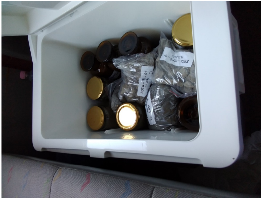
Figure 3. Collected samples are stored in mobile refrigerator (cool box)
