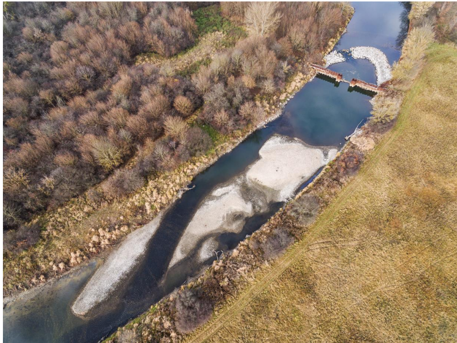
Figure 16: Partition object and example of changes of the riverbed left to spontaneous morphological development
