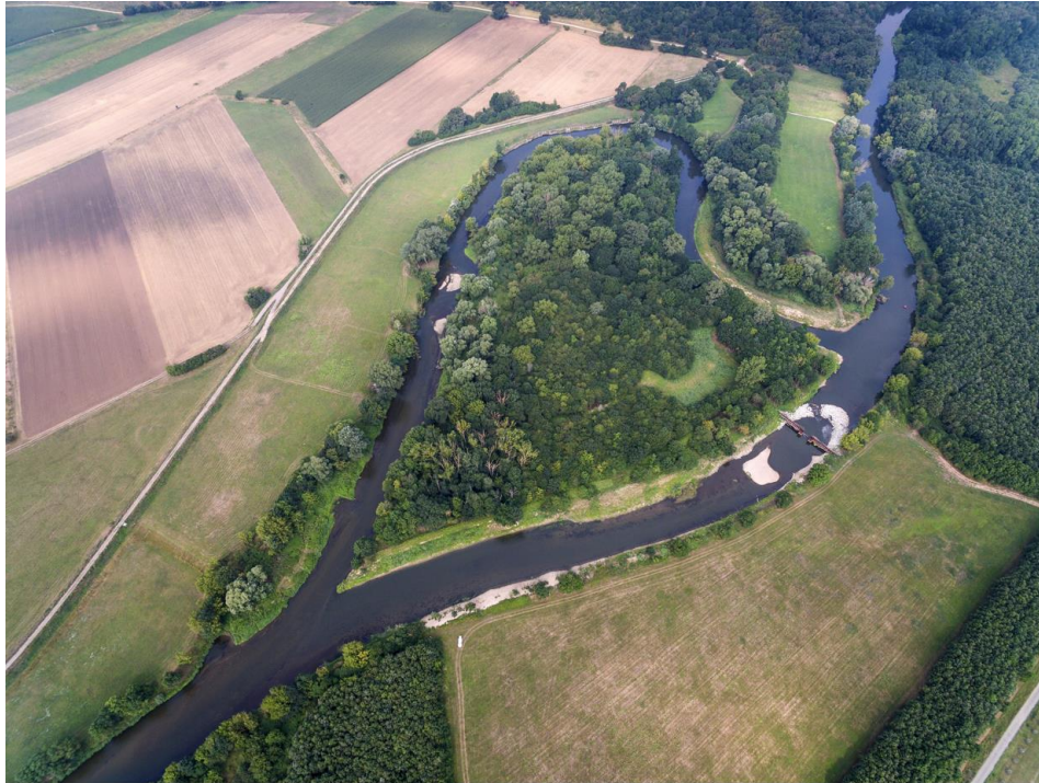
Figure 15: Restoring the orig. forcing of the riverbed - connection of the decommissioned arm on the border stream
