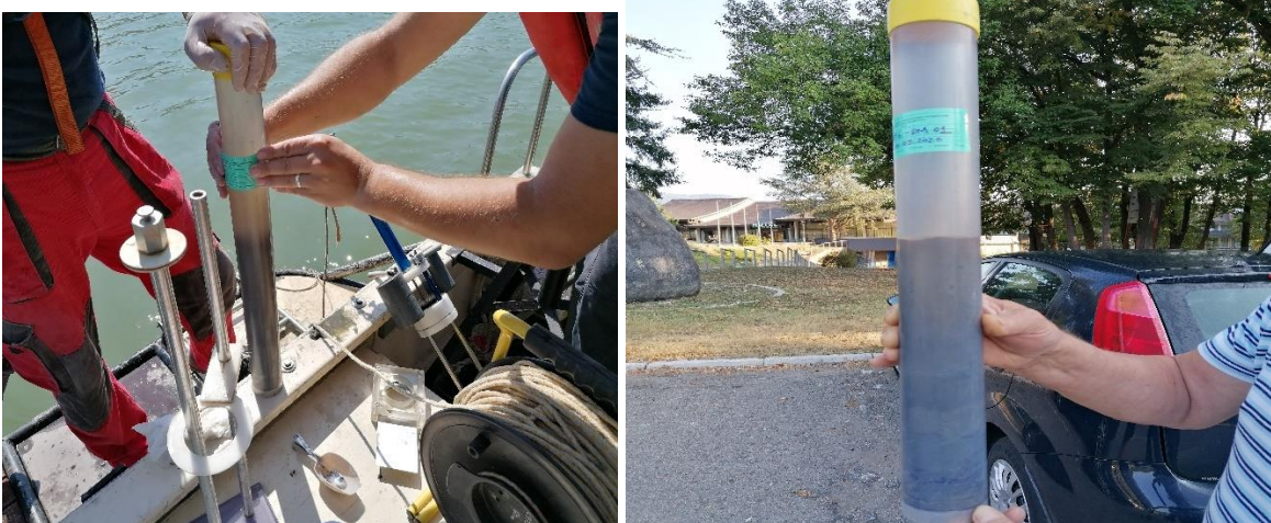
Figure 27. A sediment sample taken with a gravity corer. (Photos Marko Marjanović).
