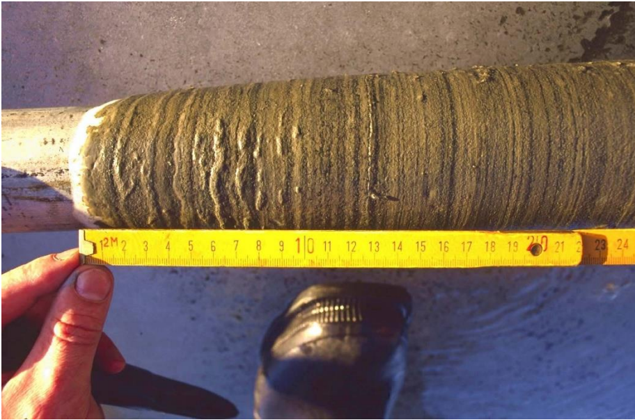
Figure 26. A sediment sample taken with a gravity corer. In this case different layers can be detected easily (Photo Seppo Knuutila).
