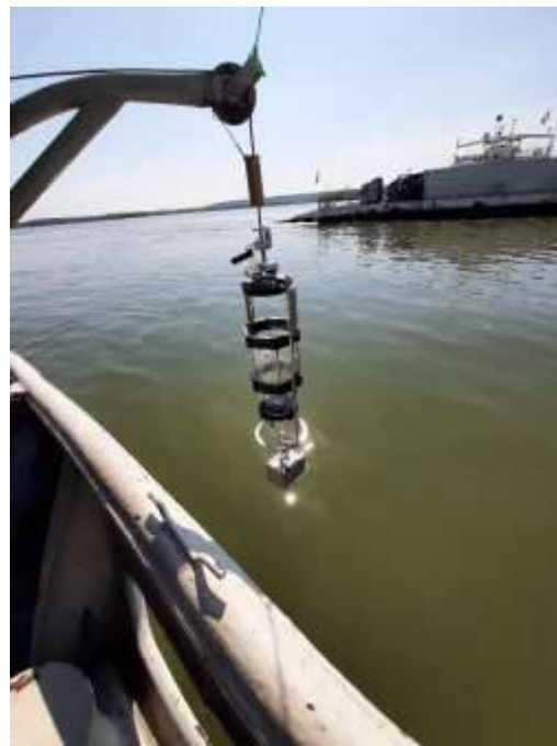
Ruttner bathometer for water properties measurements
