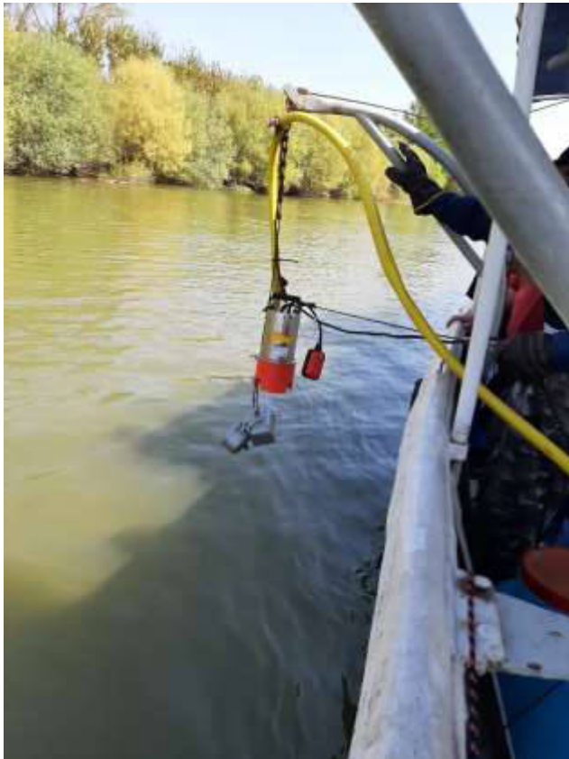
Winch for launching submersible pump
