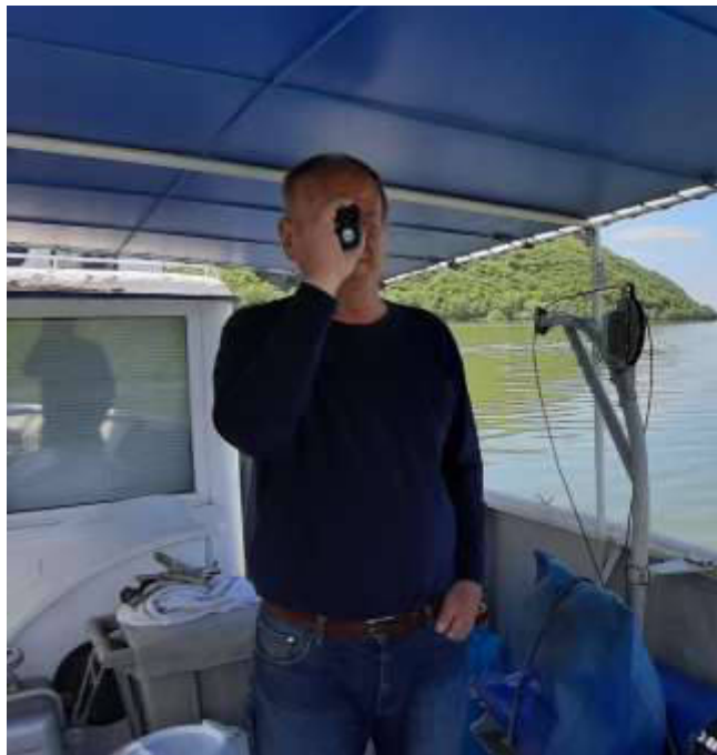
Telemeter for distance measurement between ship location and river bank
