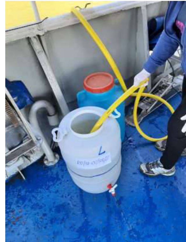
Filling one barrel with water containing suspended sediment from three depths in each vertical of the profile
