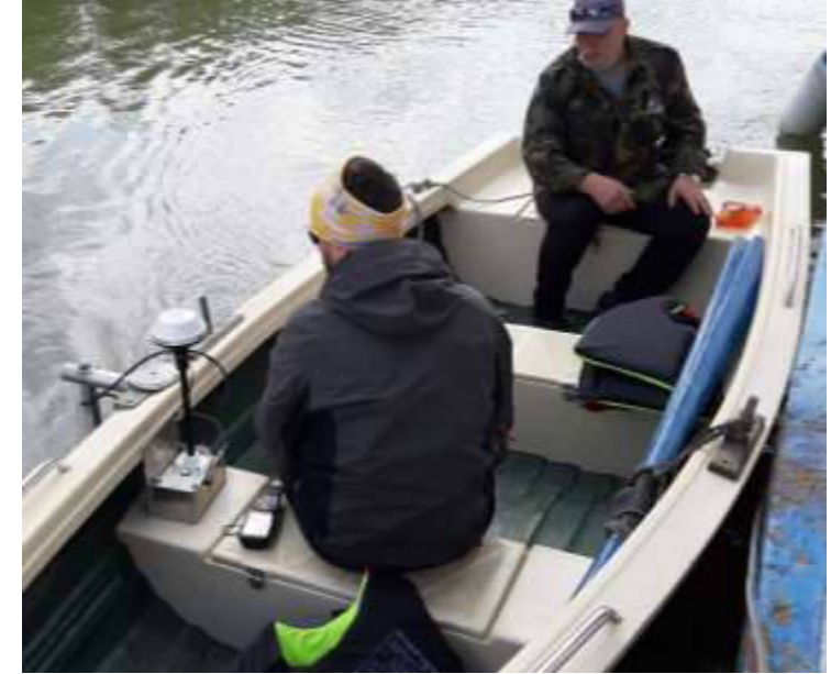
ADCP (Acoustic Doppler Current Profile) equipment for river width, depth and flow rate measurement
