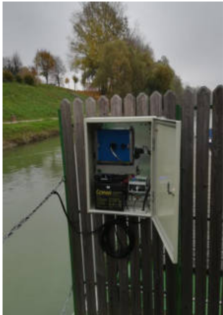
Communication box, accumulator, SIM card
