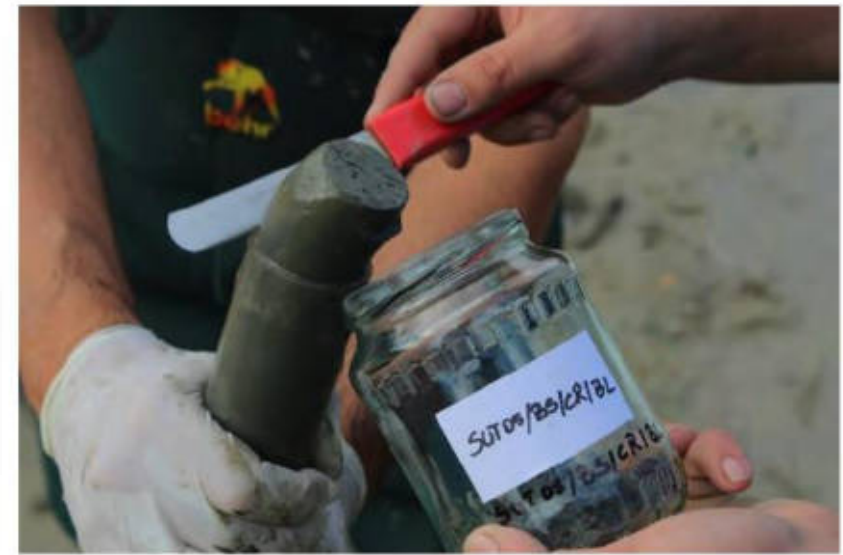
Figure 5.3. Loading jar with bottom layer sediment from the vacuum core system
