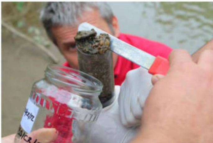
Figure 2.6. Loading jar with bottom sediment from the vacuum core system
