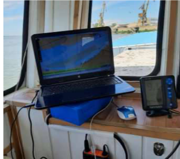
Sonar for river depth measurement on the command deck of the ship
