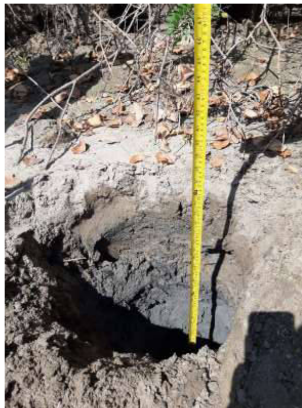
Five cm thick, dry sand topsoil, on 15 cm oxidized brownish sand covering 30 cm thick gray sandy loam
