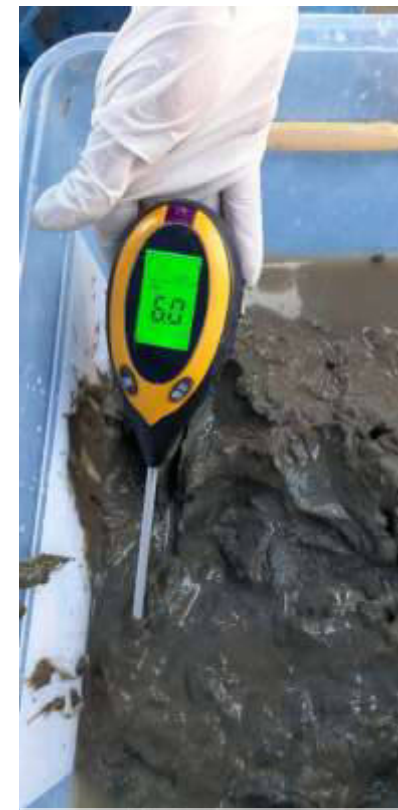
Physical properties measurements of sampled sediment (pH, temperature)
