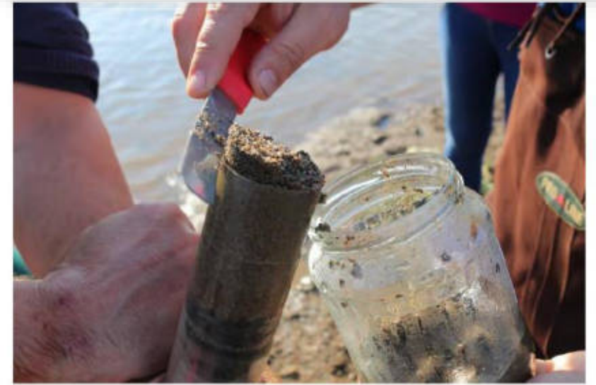
Figure 1.7. Loading a jar with bottom layer of the bottom sediment from the vacuum core system
