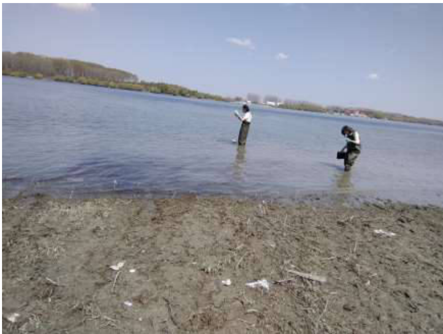
Measuring the water turbidity with Secchi disk
