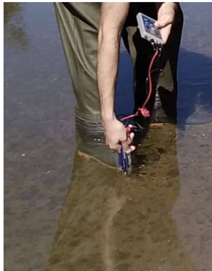
Taking in situ measurements (water pH, temperature, electric conductivity)
