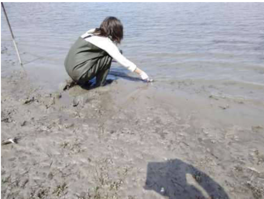
Collection of bottom sediments with a scoop
