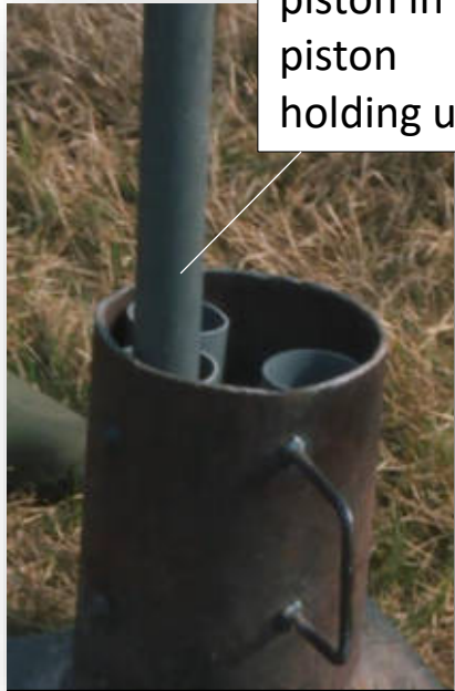
14. INSERT PISTON INTO PISTON HOLDING UNIT
