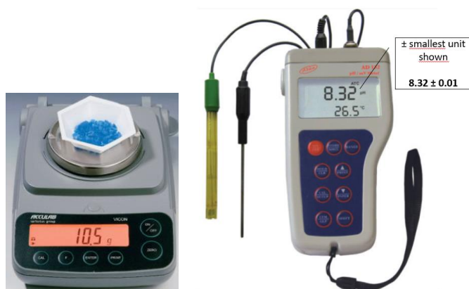
Figure 9. Uncertainty of measurement in case digital devices - examples. Digital scale (left) and digital pH meter (right).
