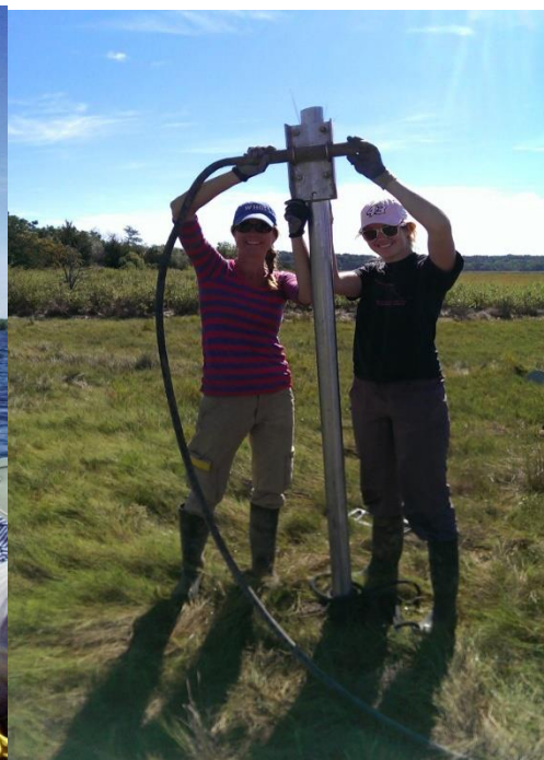
Picture 14. - Example of modern sediment corer samplers
