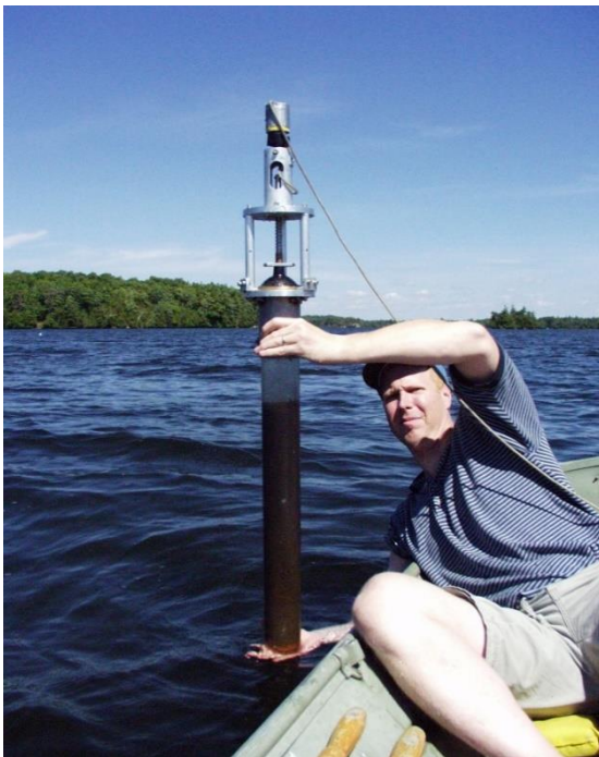
Picture 14. - Example of modern sediment corer samplers
