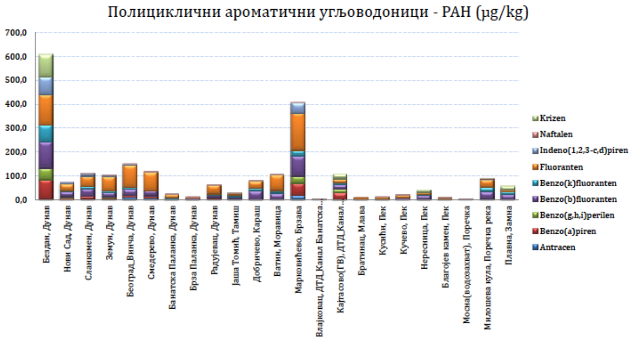
Picture 3. - The concentration of polycyclic aromatic hydrocarbons in surface waters in the Republic of Serbia
