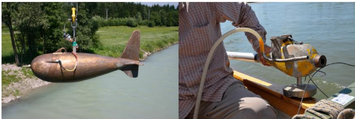
Picture 9. - Example suspended sediments samplers a) US P61 A1, b) Pump sampler
