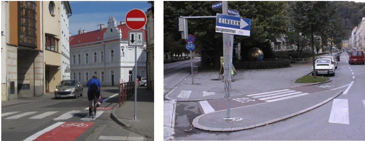
Figure 22: Contraflow cycle facilities in Czech Republic (left) and Austria (right) (Source: Danube Cycle Plans and KfV)
