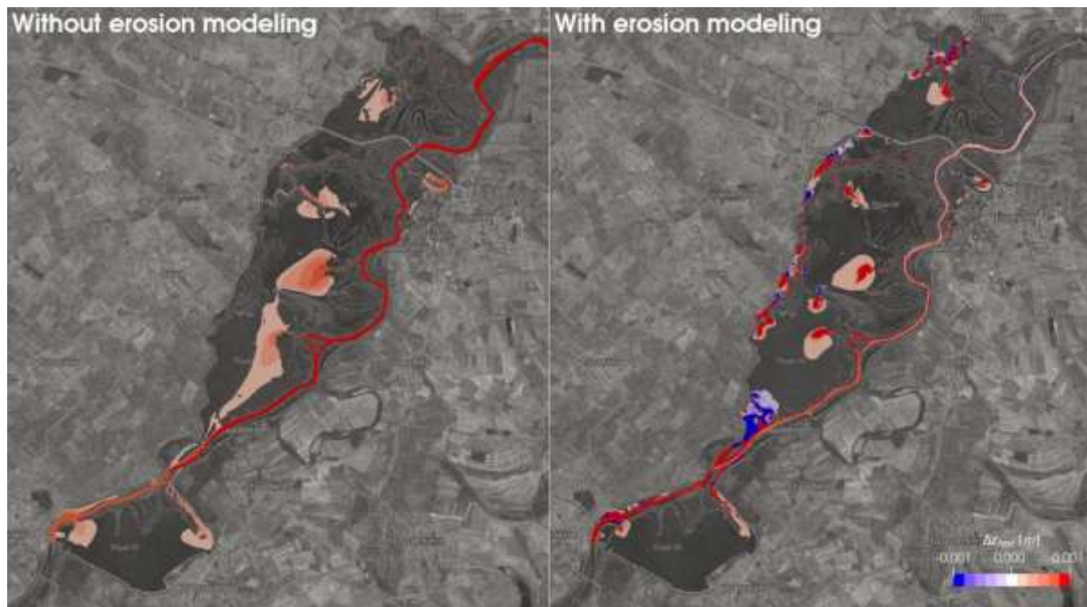
Figure 23 Comparison of final bed level change without (left) and with (right) erosion modeling.
