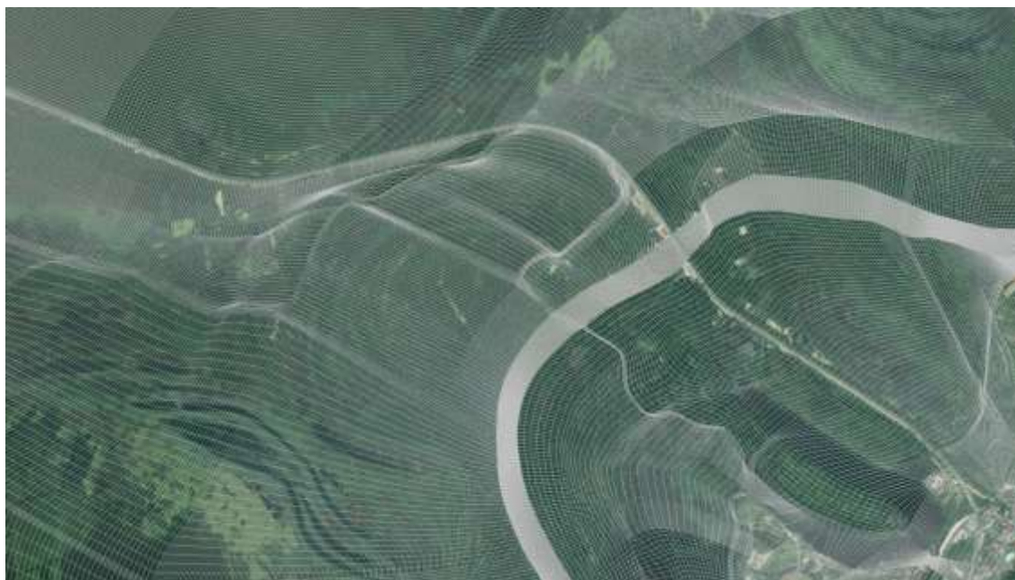
Figure 3 Section of the computational grid with an orthophoto as background.
