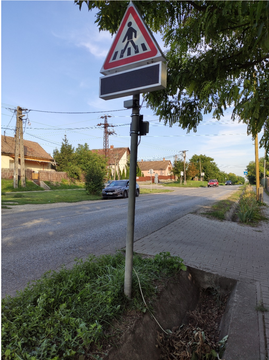
Figure 1: The pedestrian crossing warning sign with interior lighting, the LED text (Lassíts!), the first radar (looking at the same direction as the signs), and the WiFi transmitter (at the back of the pole)
