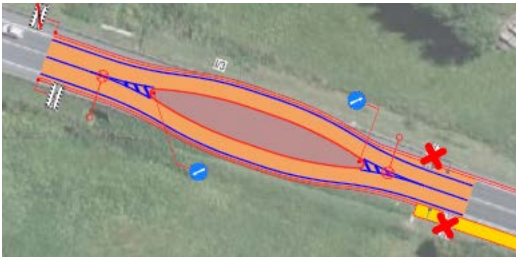
Figure 63 – Proposed safety upgrading countermeasures – entry islands
