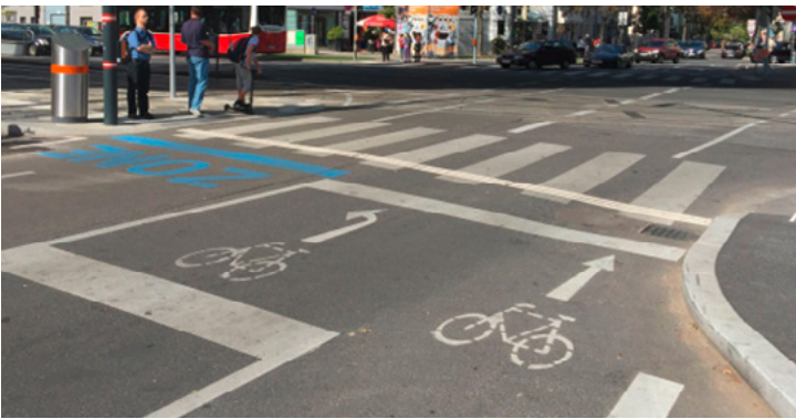
Advanced stop line (bike box) for cyclists in Vienna [12]
