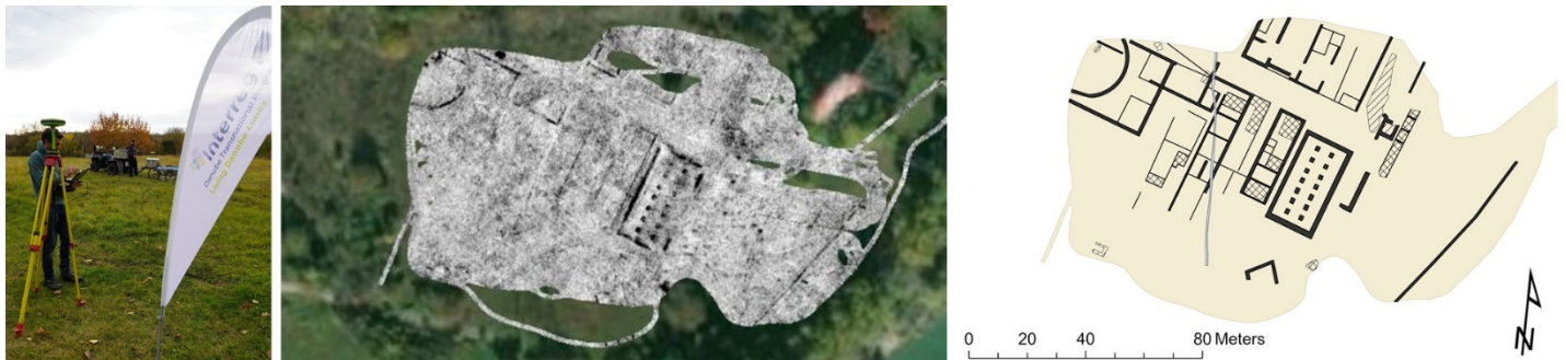
Photos by LBI ArchPro: Photo left: Setting up the GPR system at Százhalombatta; Photo middle: Survey field in the area of the Roman fortress; Photo right: Interpretation of the GPR data showing Roman building structures.
