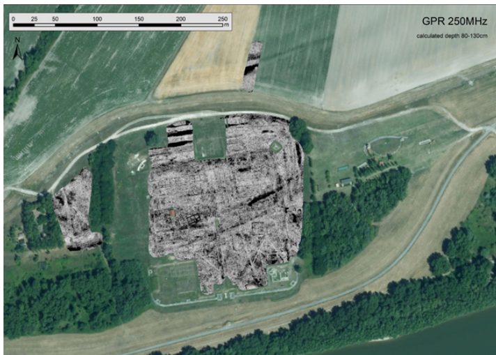
Photos by LBI ArchPro: Photo left: Overview of the GPR survey with 250 MHz antennas; Photo right: Archaeological interpretative mapping of the GPR surveys of the Roman fortress at Iža.
