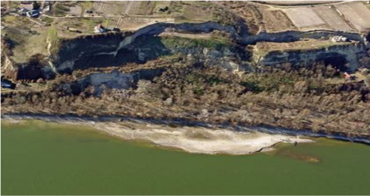
Large landslide in Dunaszekcső 30-35 meters of the river bank broke away along a 300 meter long section and slid down about 10 meters in 2008, taking with it more parts of the Roman fort of Lugio.
