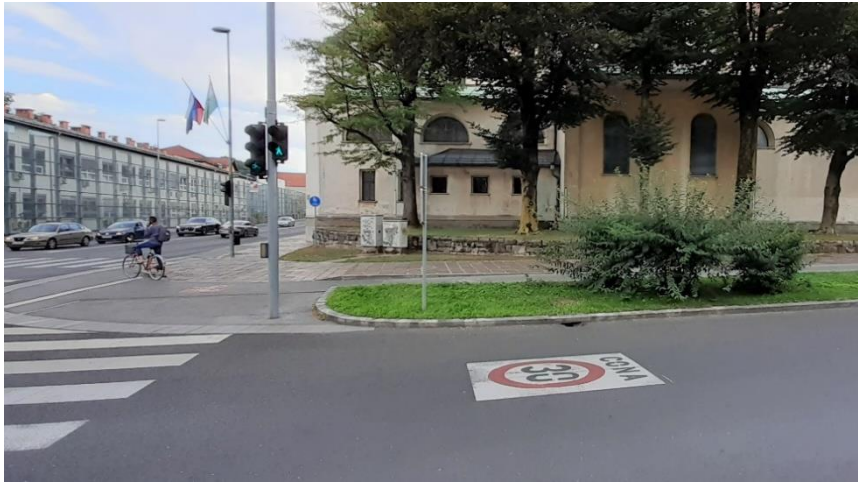
Figure 3 Road with speed limit 30 km/h is acceptable for cyclist when the traffic volume is 2000 cars/day or less
