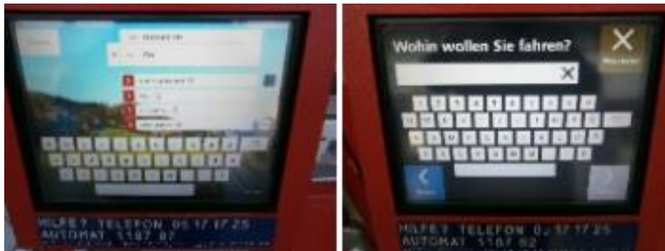
Figure 9: Ticket machine with simplified mode for visually impaired passengers at Austrian Federal Railways
