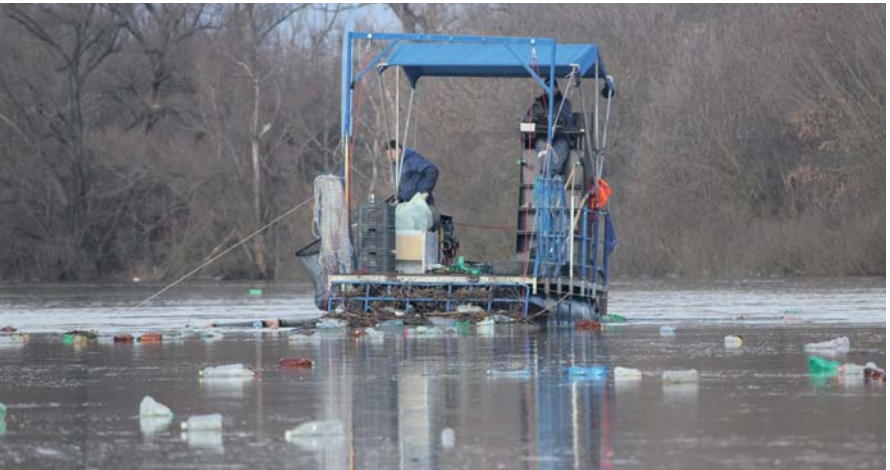
PETII, the low cost and maintenance workboat, on a winter river cleanup intervention on the Bodrog river. The arms on both sides, just like the front collector basket are detachable and can be adjusted according to the current in order to retrieve floating plastic during flood events
