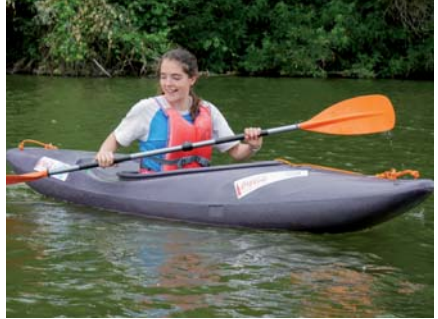
A whitewater kayak produced from selected, shredded, grinded and micronized riverine litter in the framework of the Zero Waste Tisza project.
