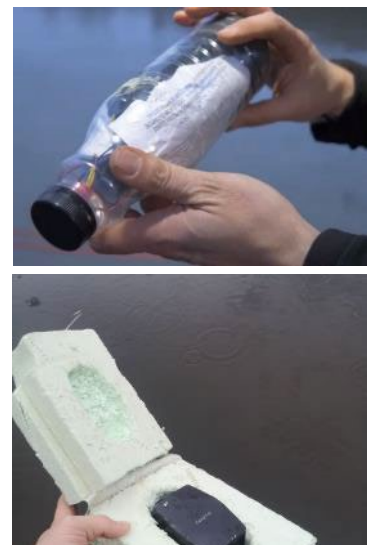
Figure 23: Used macro plastic items filled with different GPS transmitters GPS in the ongoing TidyUp field trial
