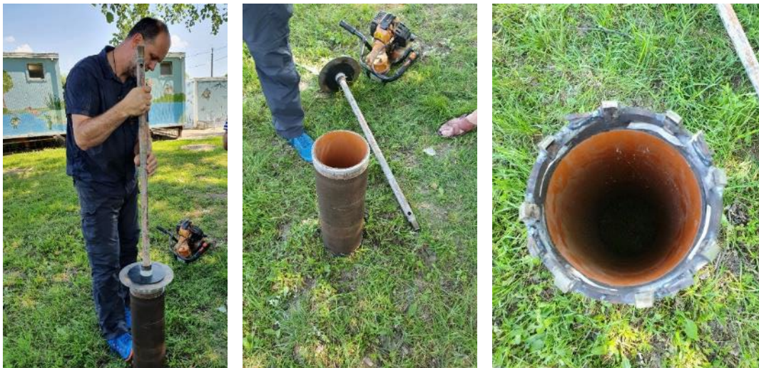
Figure 25: Prototype of sampling device for macro-plastics in fluvial sediments within Tid(y)Up project
