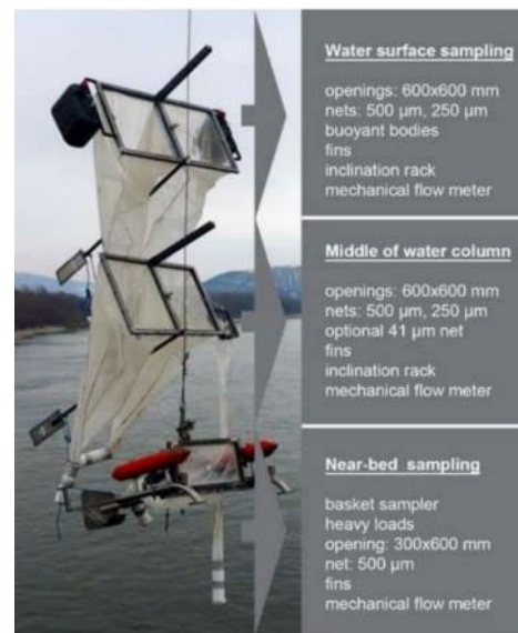
Figure 2: Net device developed by Liedermann et al. (2018).
