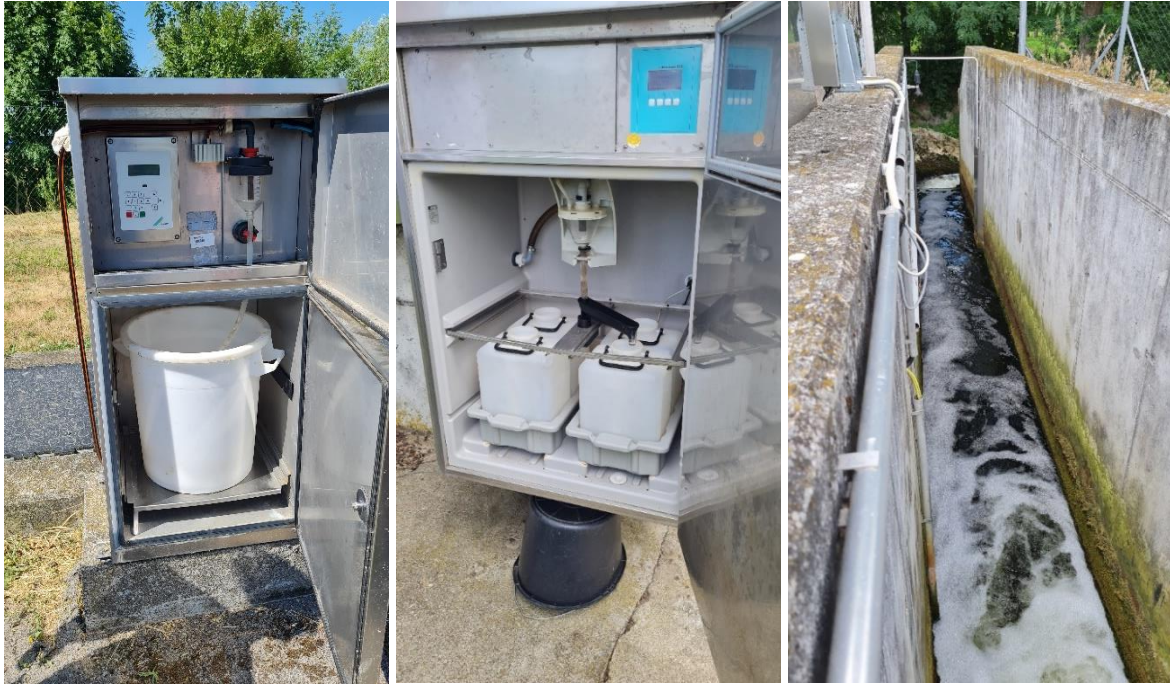
Figure 20: Sampler of effluent at WWTP A (left) and at WWTP B (middle & right) at Wulka catchment.
