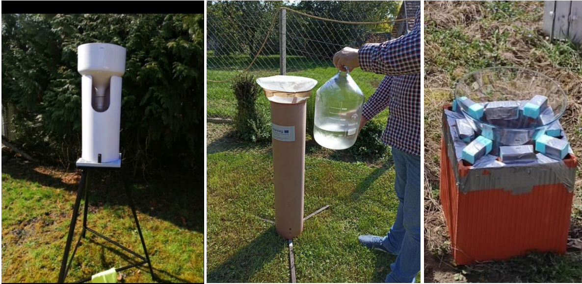
Figure 17: Examples of the applied simple deposition collectors at Viseu (left), Koppány (middle) and Vit (right) catchments.
