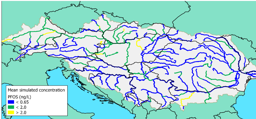
Figure 55: Simulated long term average concentration of PFOS as a result of present emissions.
