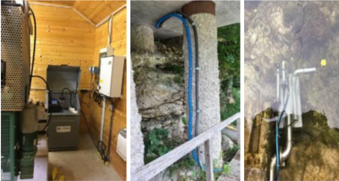
Figure 11: Autosampler and probe arrangement at Opponitz station (Upper Ybbs, AT).
