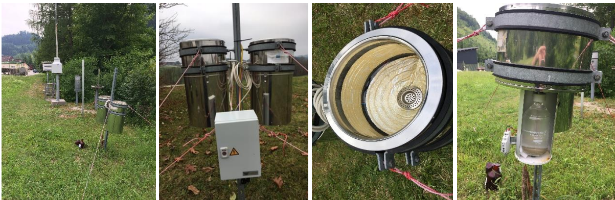
Figure 18: Atmospheric deposition samplers and transformer at Krenstetten and at Opponitz.
