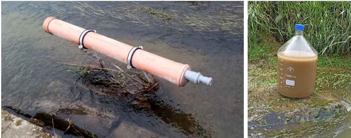
Figure 15: Philips type sampler for high-flow condition at Nemti station (left) and sample collected from a flood event at Törökkoppány station (right).
