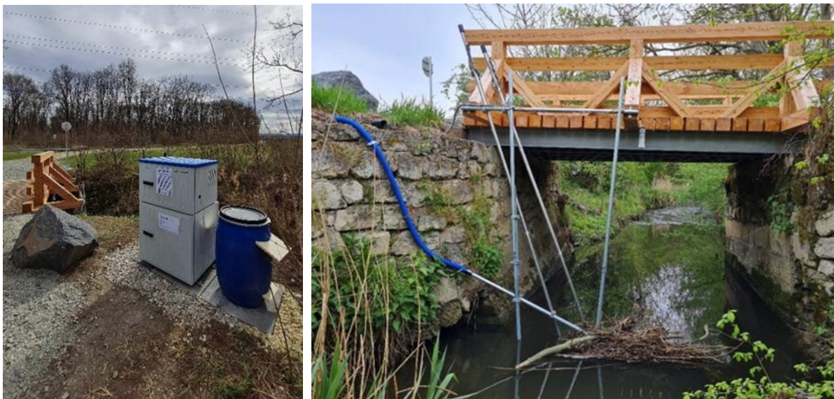
Figure 10: Autosampler and sampling setup at Eisbach station (Wulka, AT).
