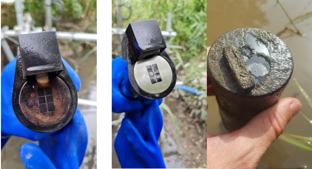
Figure 13: Turbidity sensor before and after cleaning (left) and probe with self-cleaning windows.
