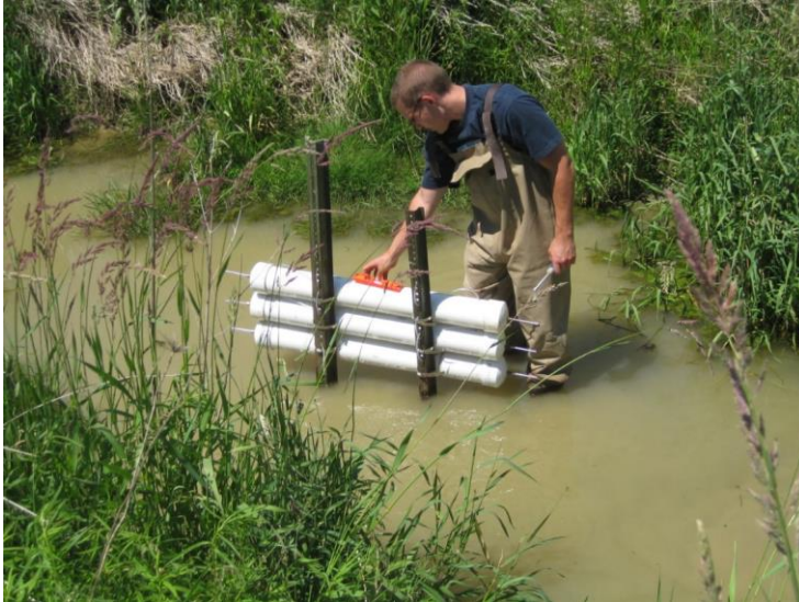
Figure 14: Time-integrated Philips sampler installation to measure different stage intervals .
