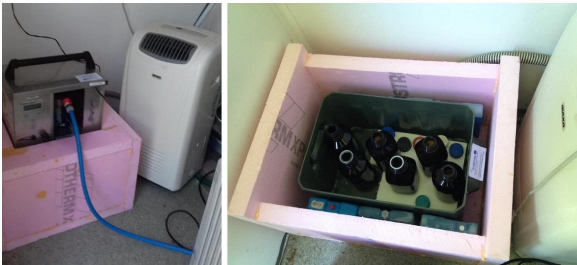
Figure 6: Passive cooling of portable sampler .
