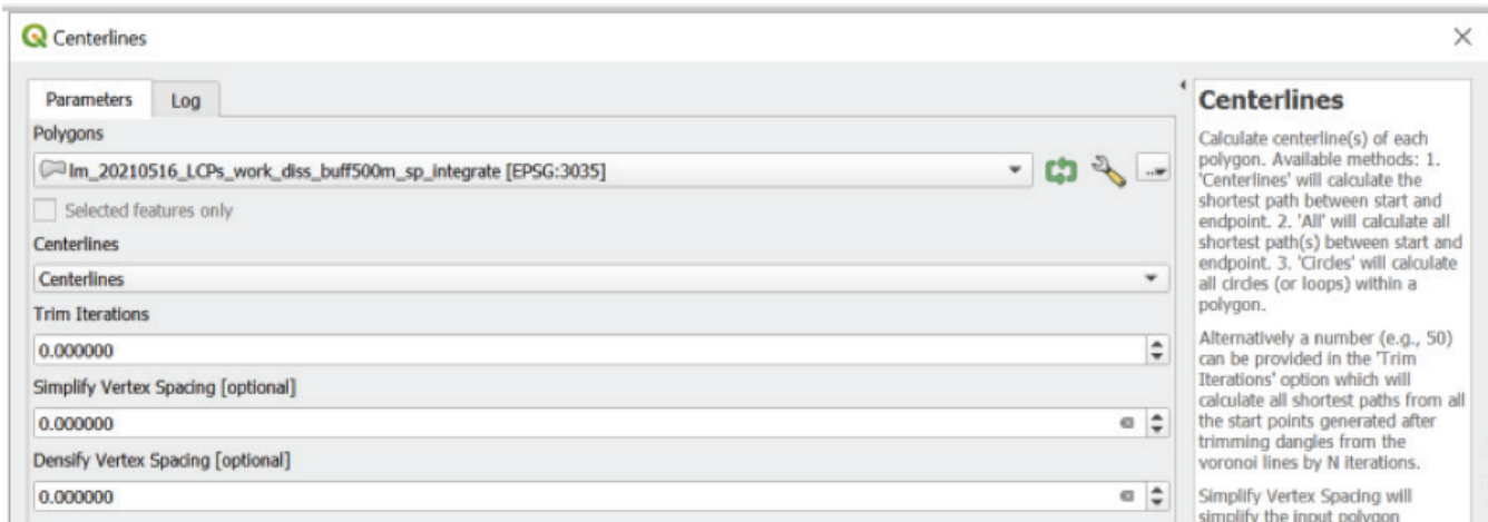
▲ Figure 27: Screenshot of the initial step of applying the “Centerlines” tool in QGIS
