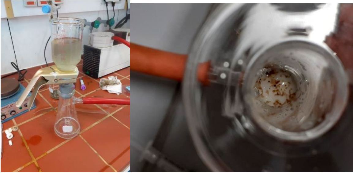
Figure 59: Vacuum-filtration of the samples (left: whole device, right: view from above of the Anodisc-filter including filter cake)
