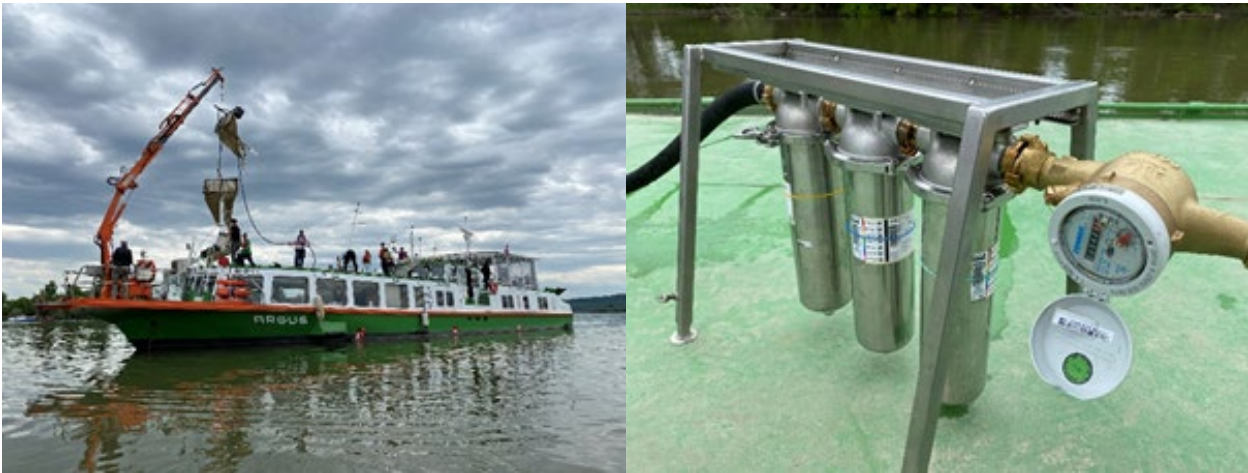
Figure 39: Argus ship with net device and suction pump on the Danube River, Pančevo (RS)
