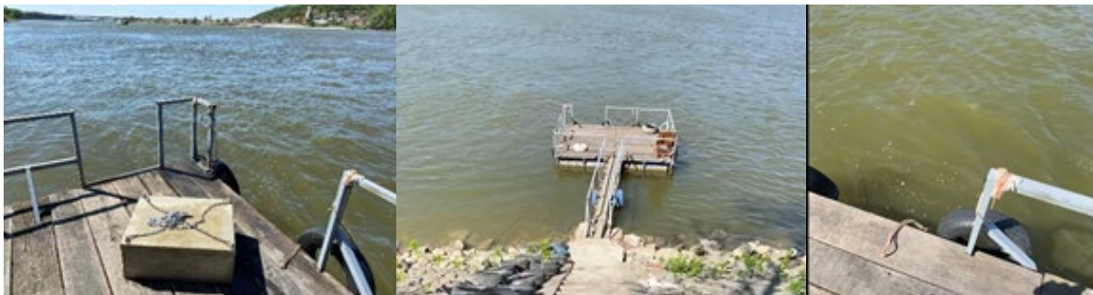
Figure 34: Deployed sedimentation box in Bezdán (RS)
