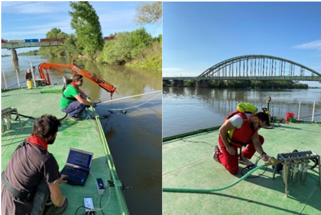
Figure 48: Microplastic sampling using net device and suction pump on Argus ship – Tisza River (Titel, RS)
