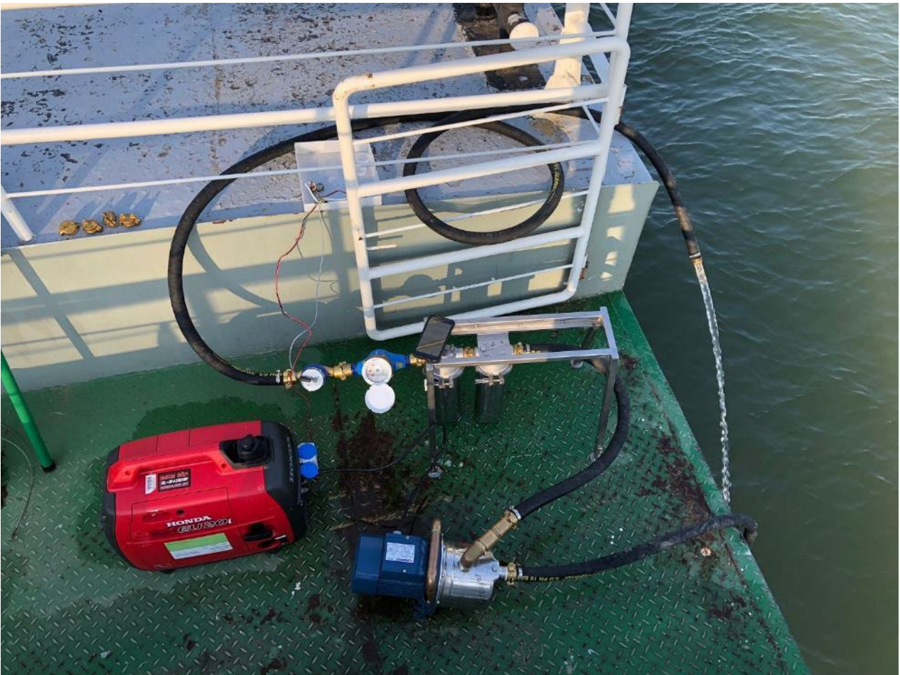
Figure 19: Fractionated filtration device in use.
