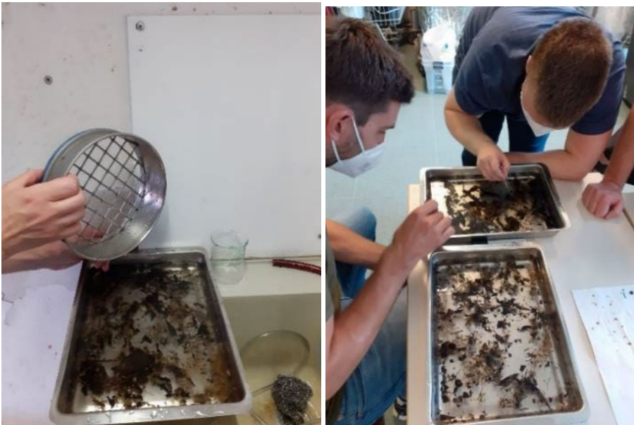
Figure 54: Removal of macro plastics and visually picking of microplastics (mesh size: left > 20 mm, right 5 mm-20 mm)
