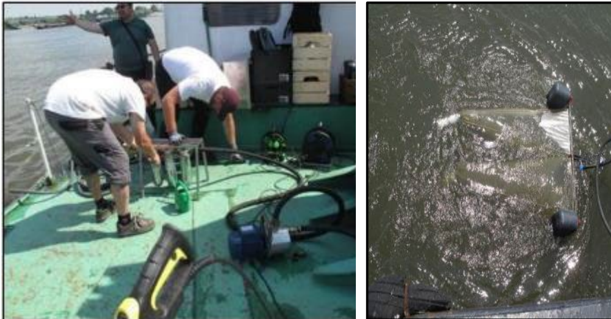
Figure 43: MP Sampling with net and pump devise in Ruse, BG
