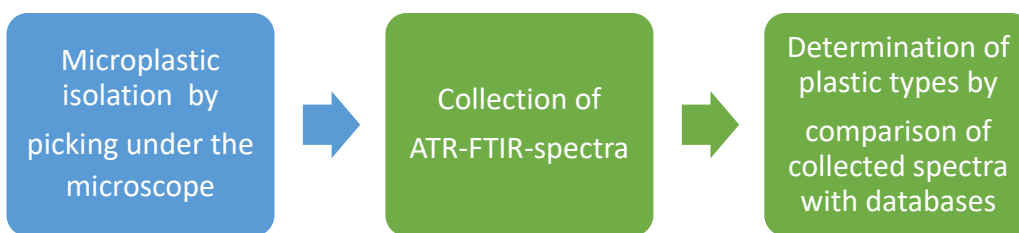
Figure 58: Analytical procedure size class 1000-5000 \mu\text{m}
