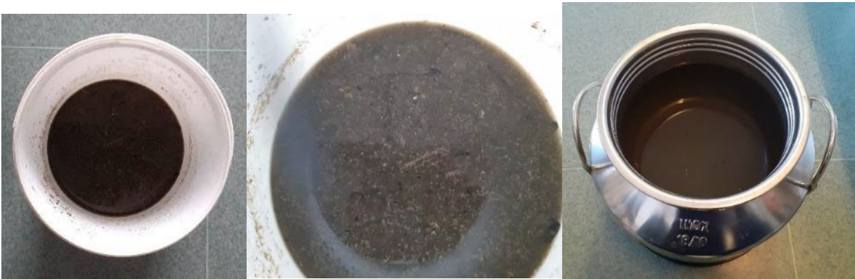
Figure 51: Examples of samples (left, middle: samples taken with net; right: sample taken with sedimentation box)
