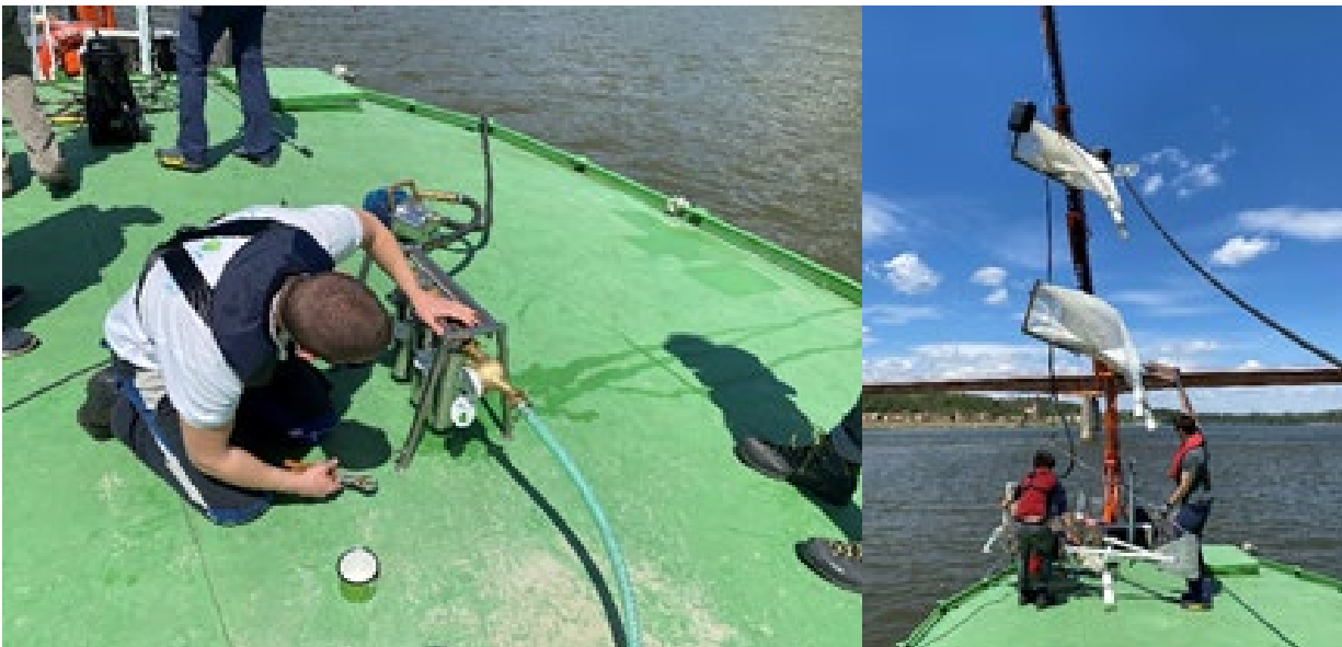
Figure 36: Suction pump and net device sampling, Bezdán (RS)
