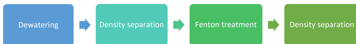
Figure 65: Sample pre-treatment steps of sedimentation box samples
