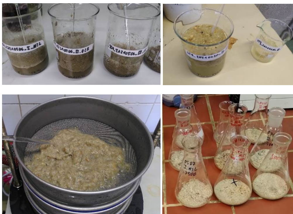
Figure 55: Samples before digestion of organics (above left), after Fenton treatment (above right); after treatment, during sieving (below left) and after sieving and oven dried (below right)
