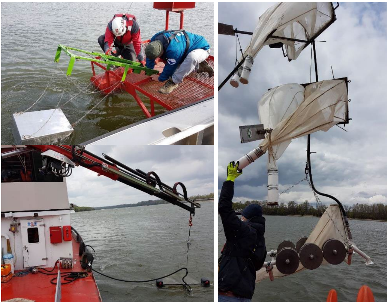
Figure 30: Deployment of the sedimentation box at Budapest (top left); parallel application of the fractionated filtration and the net device (bottom left & right);
