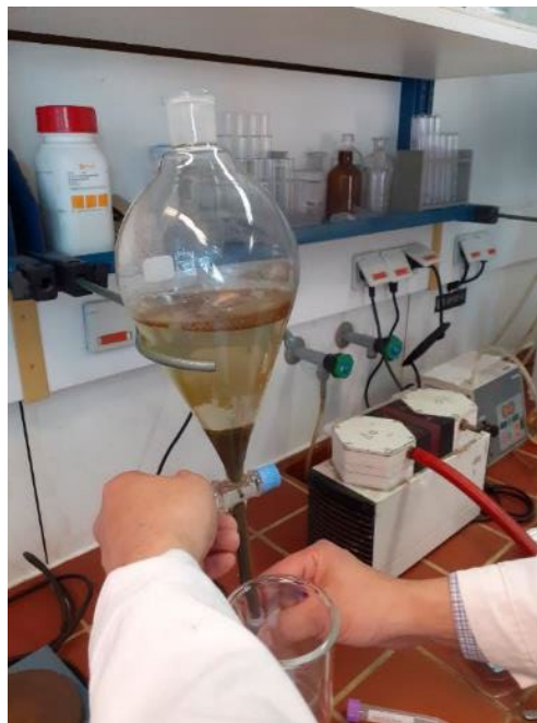
Figure 57: Density separation in \text{ZnCl}_2 -Solution (1.7 kg/l)
