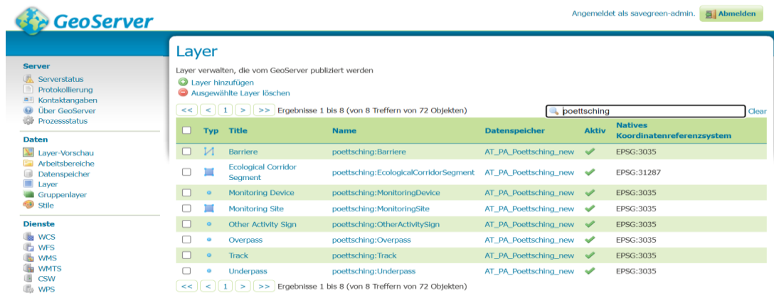
Figure 33: Adminstartion interface of the open source technology Geoserver which is used for the provision of the OGC web services
