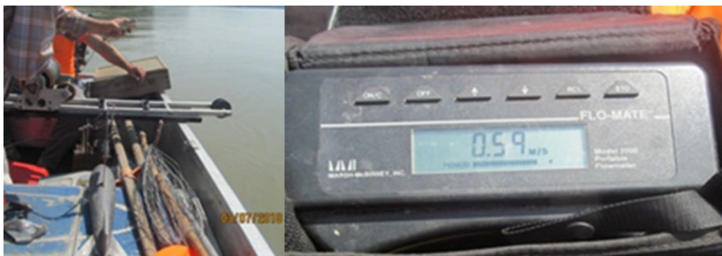
Figure 55 Portable Flow-meter FLO_MATE Model 2000 used for measurement of water velocities close to the bottom of the river (photo credit: DDNI).
