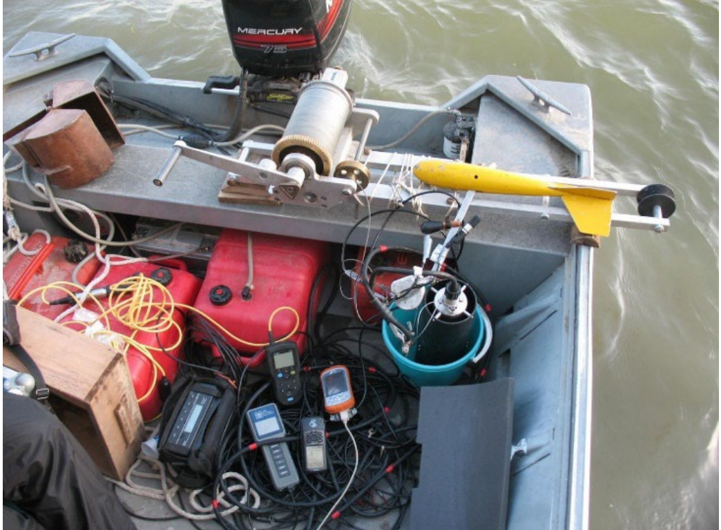
Figure 57 EFM setup to operate from the back of aluminium boat SAM (photo credit: DDNI).
