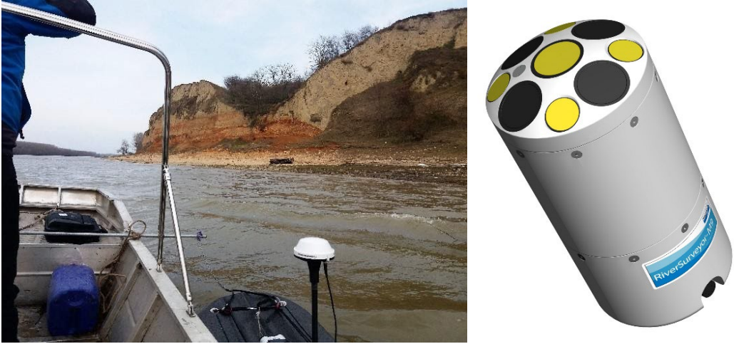
Figure 60 Left: Specifications and operation setup of River Surveyor M9 while recording current profiles at Red Rock spawning site for sturgeons in the LDR at km 311 (Source: DDNI); Right: Sontek M9 with 9 beams (photo credit: https://www.sontek.com/riversurveyor--s5-m9 )
