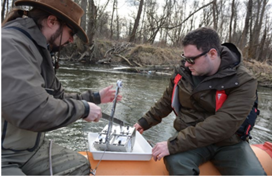
Figure 52 Using Van Veen grab (photo credit: REVIVO, 2019).
